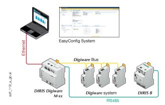
Configure the entire system with an Ethernet connection to a DIRIS Digiware D-xx display
