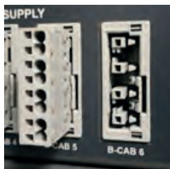
Figure 13. B-Cab aux supply connectors
