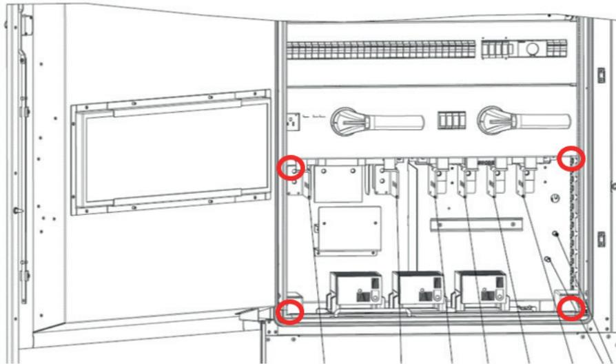
Figure 47. Screws of the plastic panel
