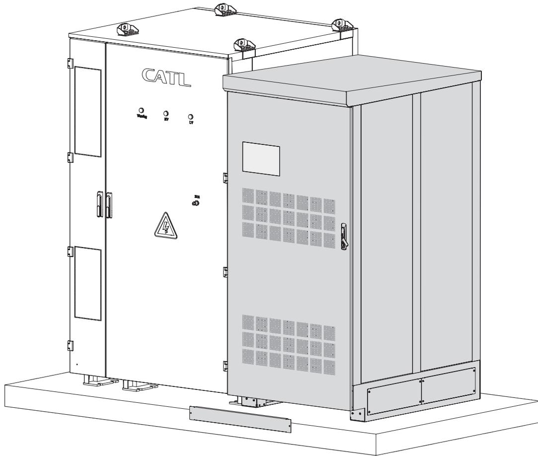
Figure 37. C-Cab front panel removal
