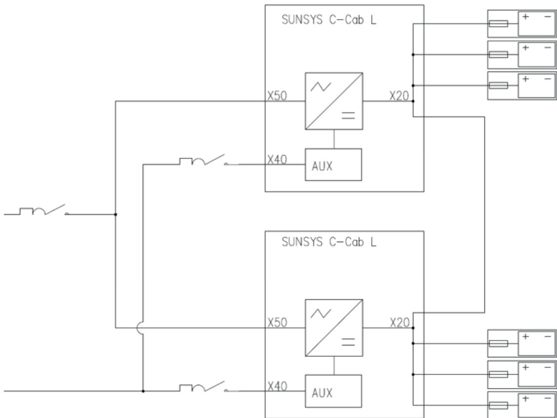
Protection of 2 C-Cabs with common AC protection (allowed) with DC-Cab
