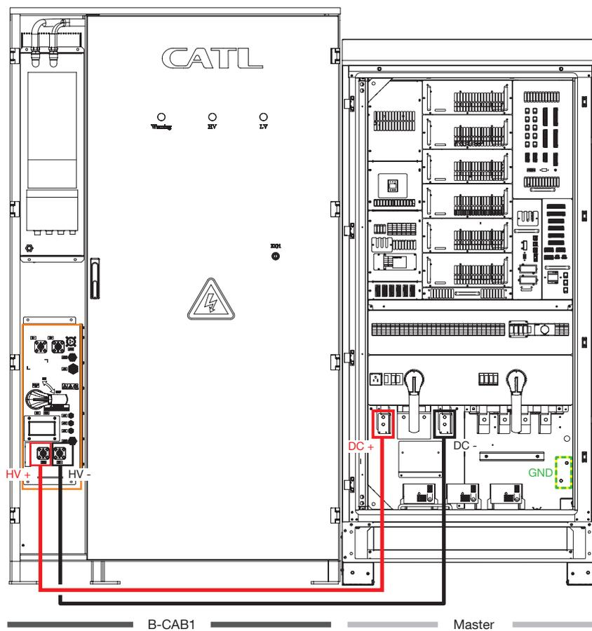
Figure 50. DC Power connections
