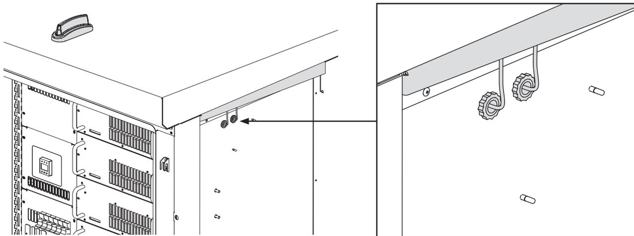
Figure 67. Cable direction from antenna to inside the C-Cab
