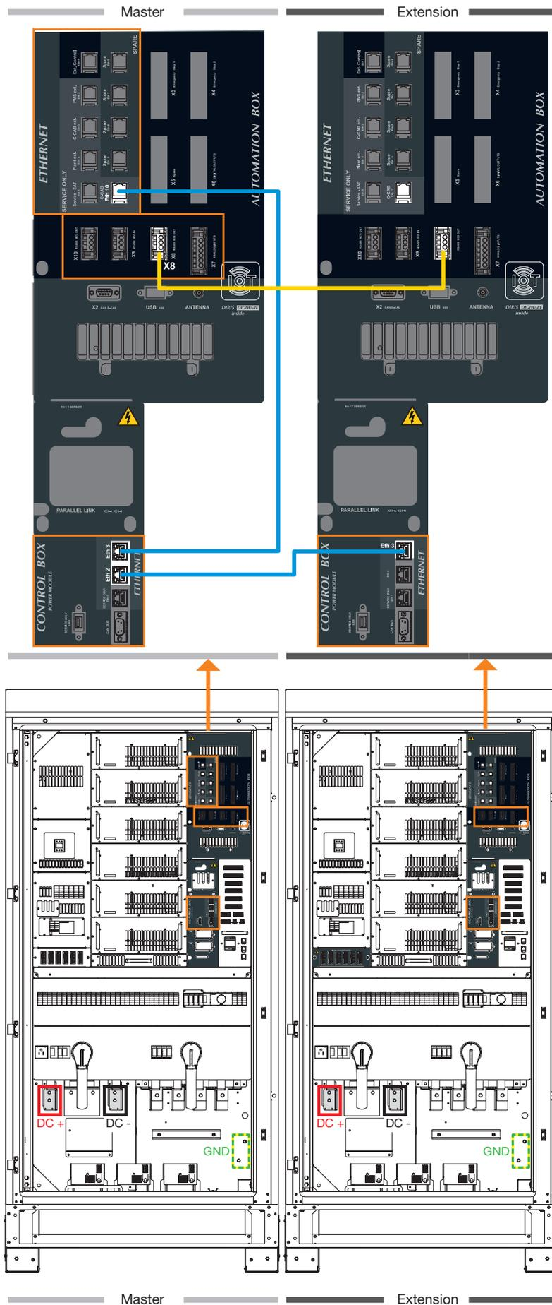
Figure 62. Figure 66 - Connection of the communication for the Digiware package
