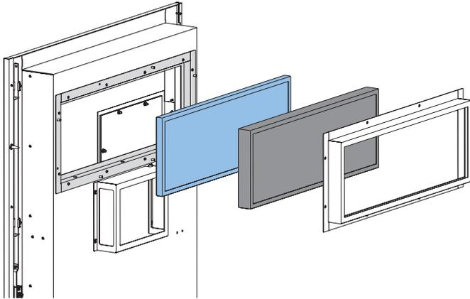
Figure 81. Installation of the air filter
