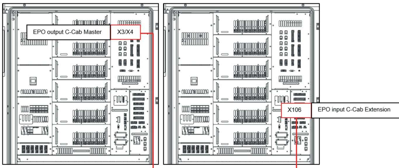
Figure 63. Location of the Emergency Power Off connections
