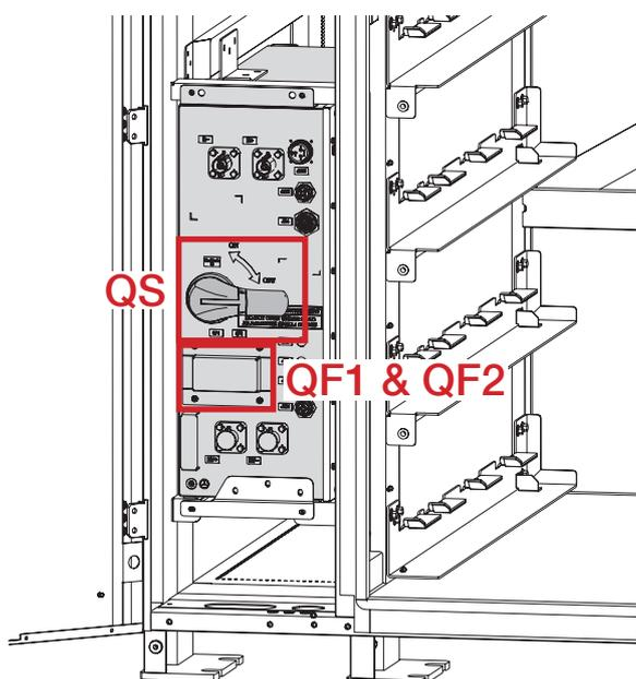
Figure 46. Location of isolation switch QS and breakers QF1 & QF2
