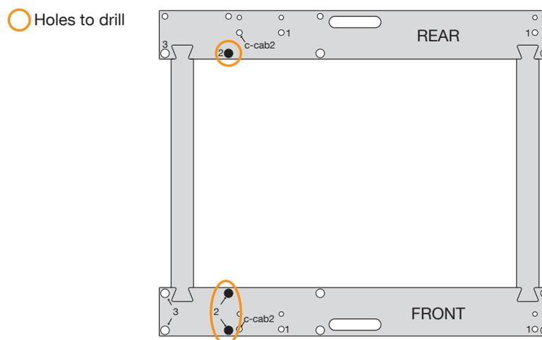
Figure 36. Holes to prepare B-Cab installation next to the C-Cab.
