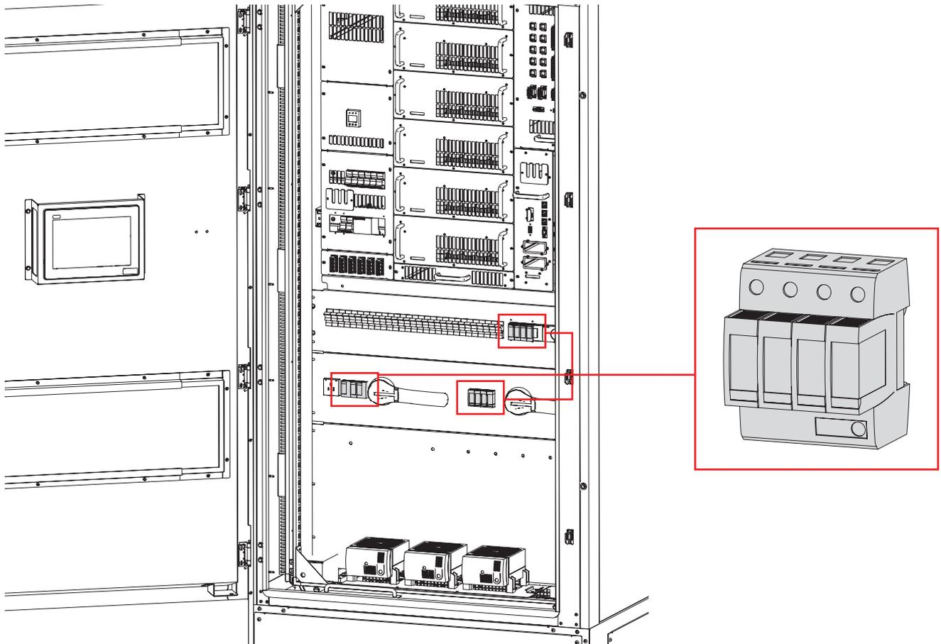
Figure 82. Location of the SPDs inside the C-Cab
