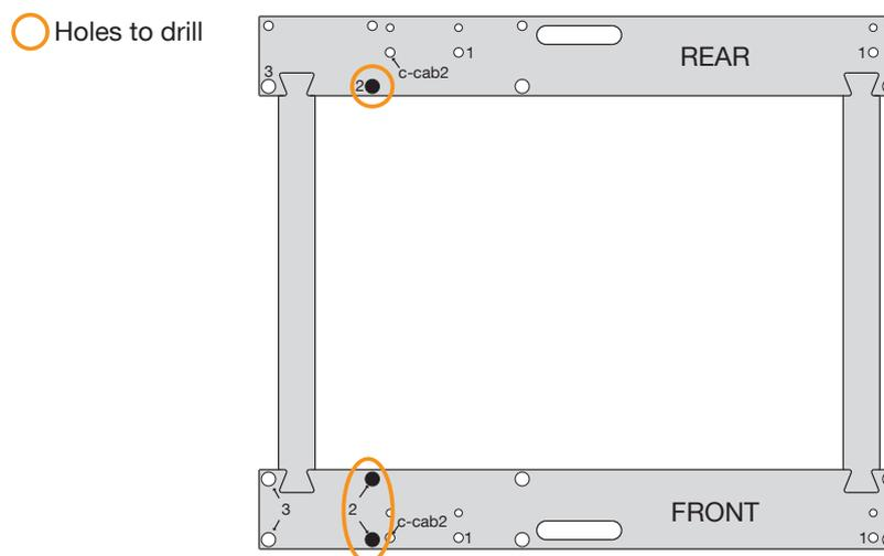
Figure 31. Holes to prepare B-Cab installation next to the C-Cab
