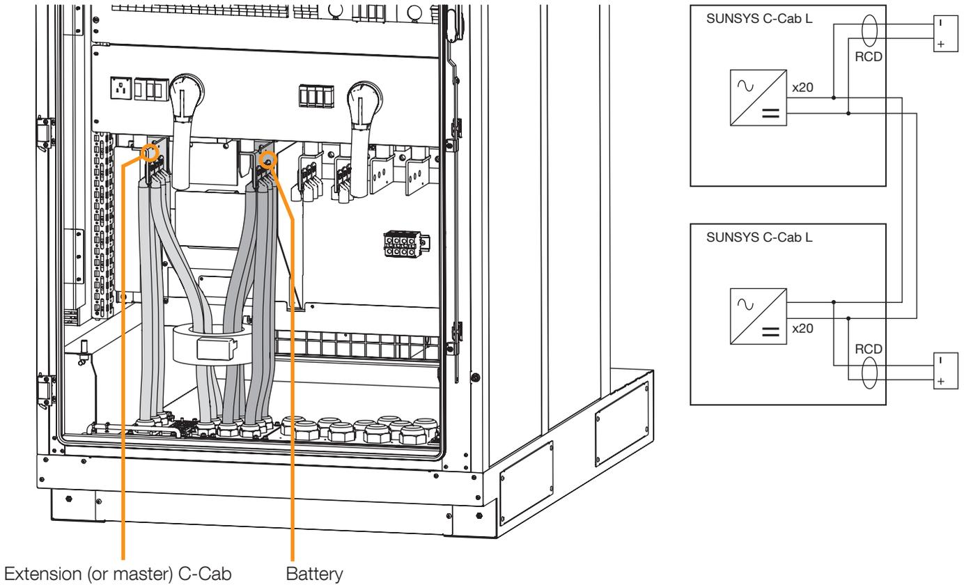
In order to allow an easier installation of the cables, start fixing the cables from the left to the right. Take care that the cables do not press too hard against the plastic of the component. Pay attention not to damage the cable connected to the RCD component during the installation.
