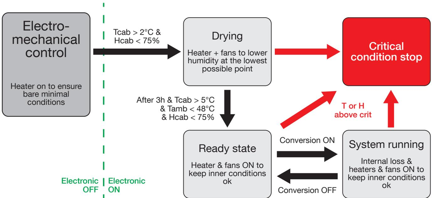
Figure 12. Environmental logic diagram
