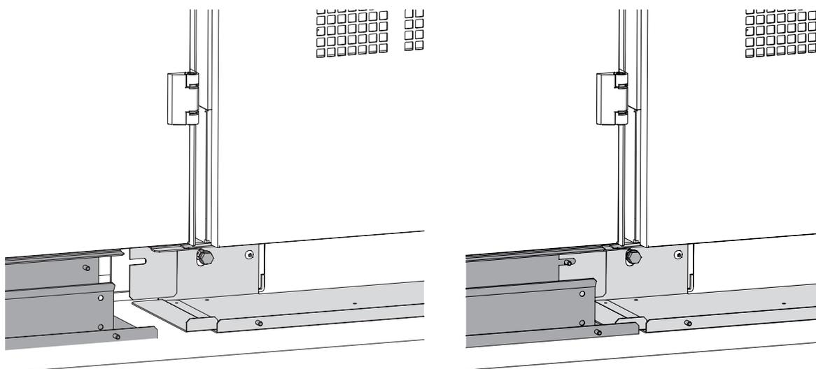
Figure 42. Connection of C-Cab and B-Cab parts
