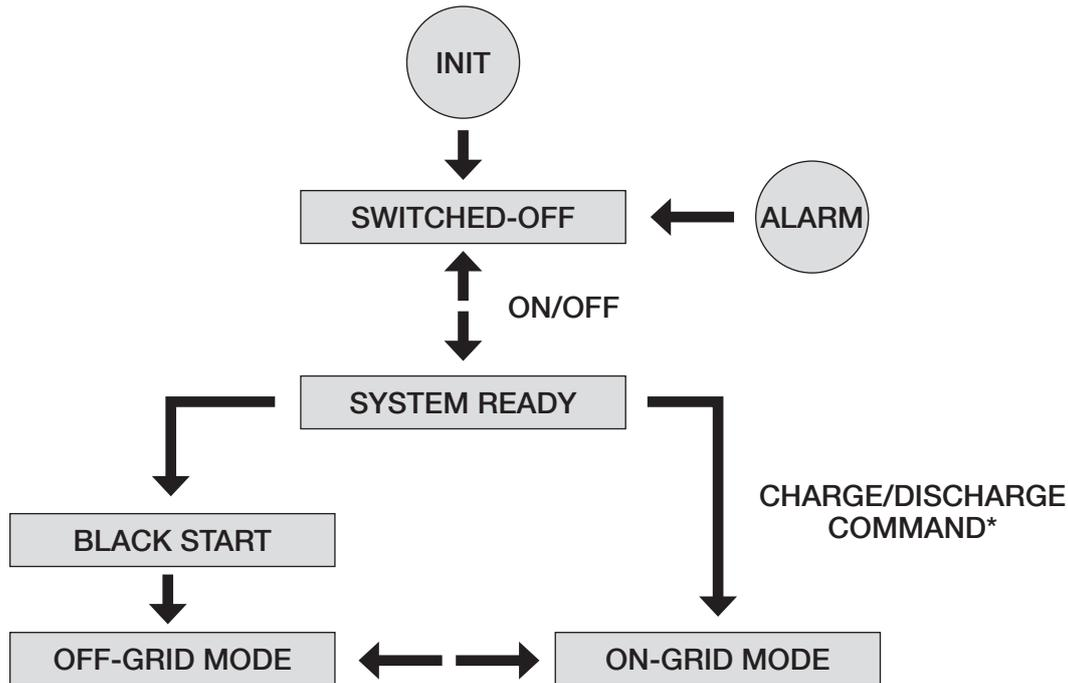
Figure 10. Modes of operation of SUNSYS HES L
