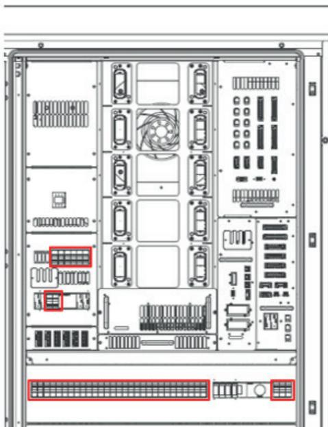
Figure 64. Location of the fuses inside the C-Cab
