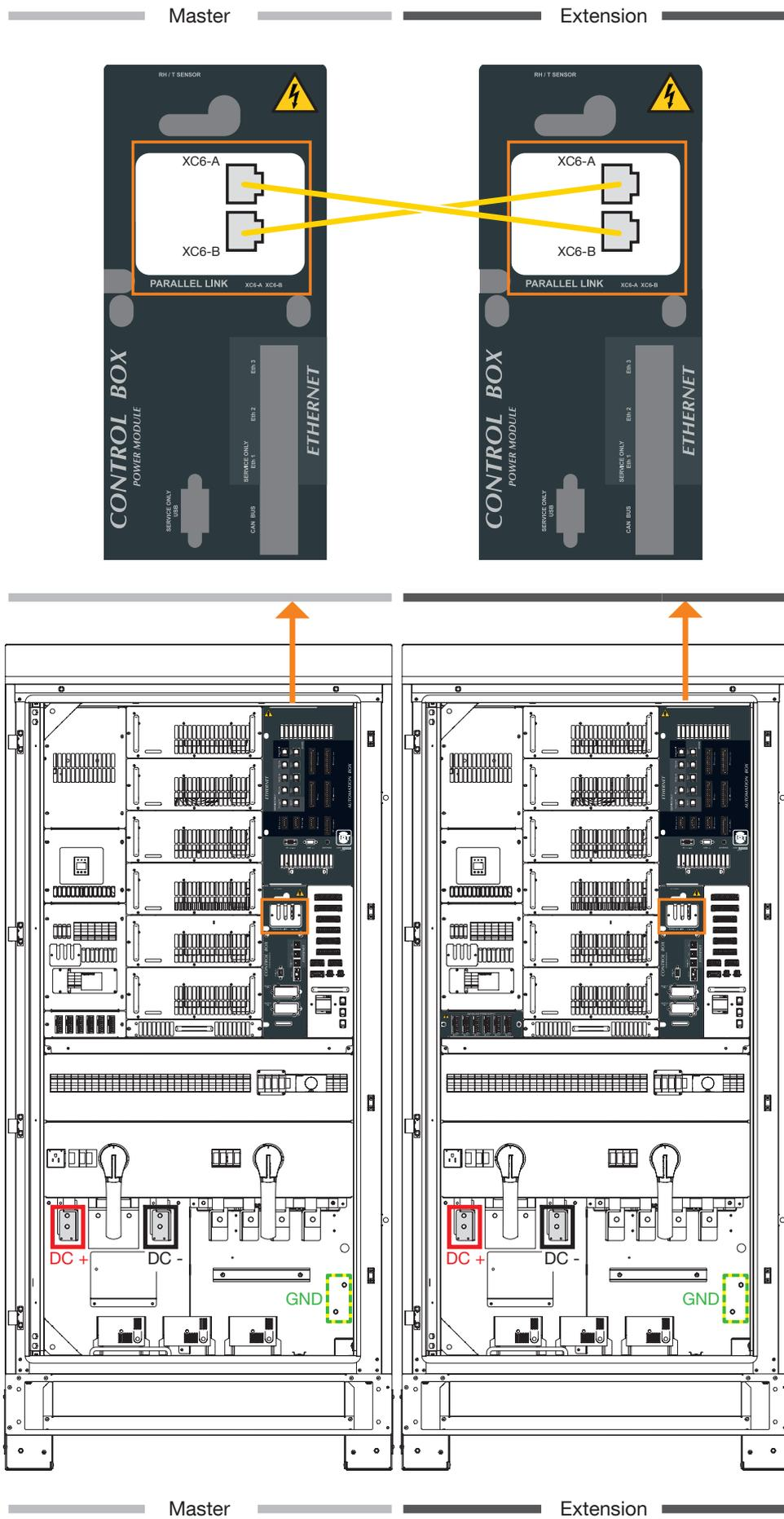
Figure 61. Connection of the communication for the paralleling
