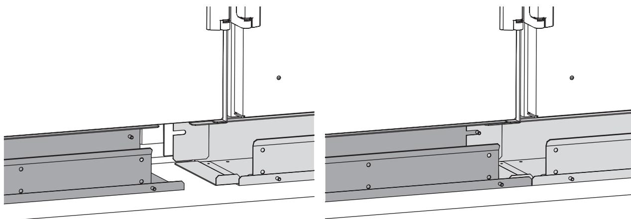
Figure 43. Connection of two B-Cab parts
