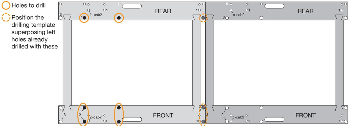
Figure 32. Holes to drill for the B-Cab installation
