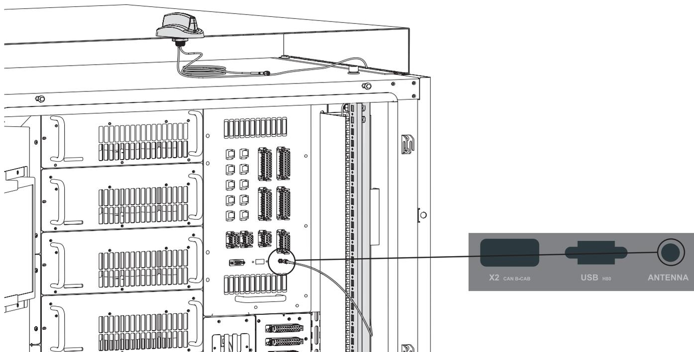
Figure 68. Connection of the antenna cable inside the C-Cab
