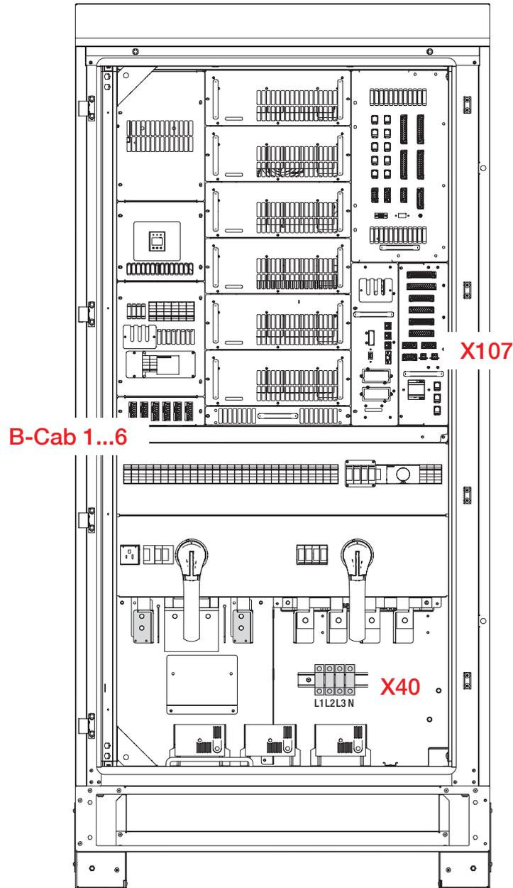
Figure 52. Location of the auxiliary connections in the C-Cab
