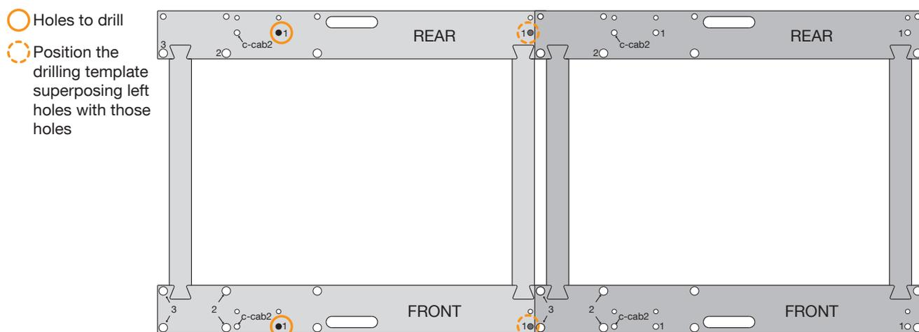
Figure 35. Holes to drill for the C-Cab installation
