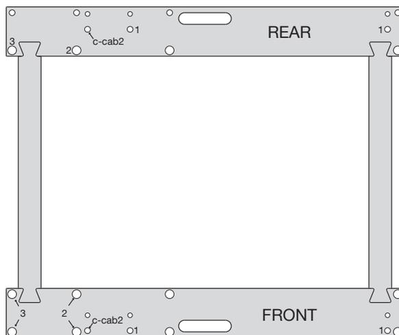
Figure 29. Top view of the drilling template mounted
