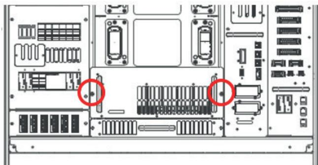
Figure 76. Power module screws location
