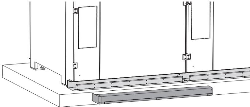
Figure 69. Screwing of the covers
