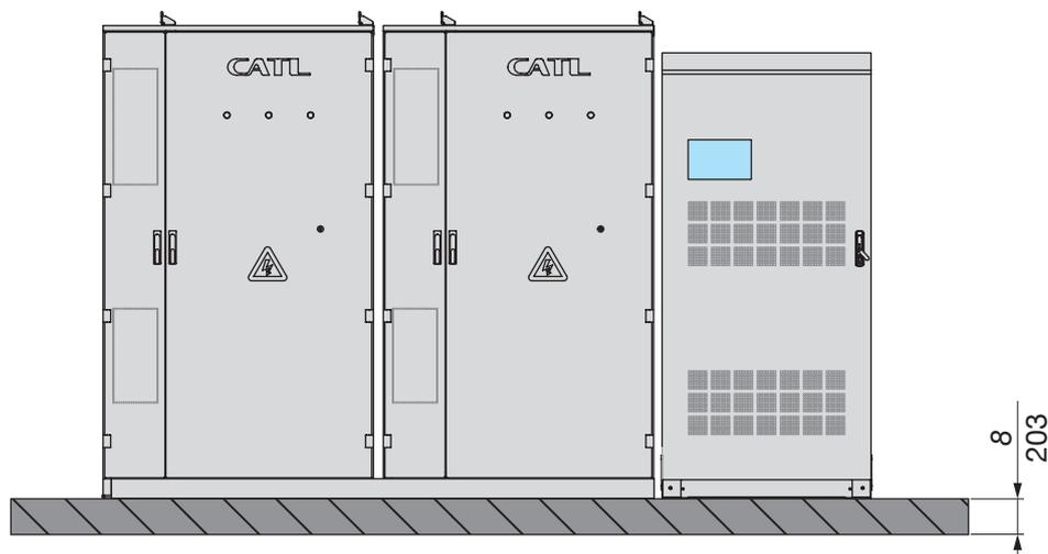
Figure 23. Concrete depth – SDS 2.5
