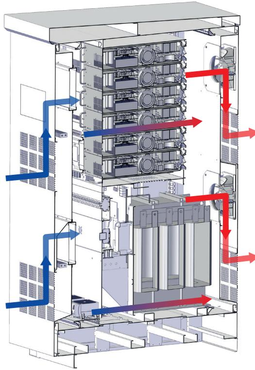
Figure 11. Air flows inside the SUNSYS C-Cab L
