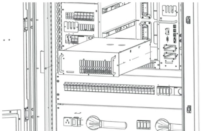
Figure 77. Insertion of the power module
