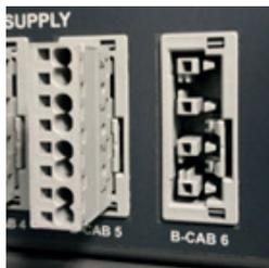
Figure 14. B-Cab aux supply connectors
