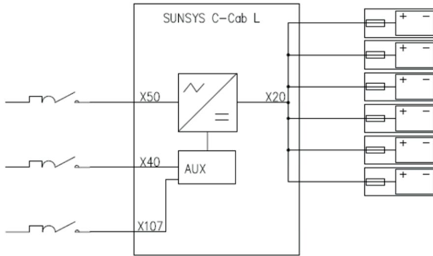
Protection of 2 C-Cabs with 2 separated AC protections (suggested) without DC-Cab
