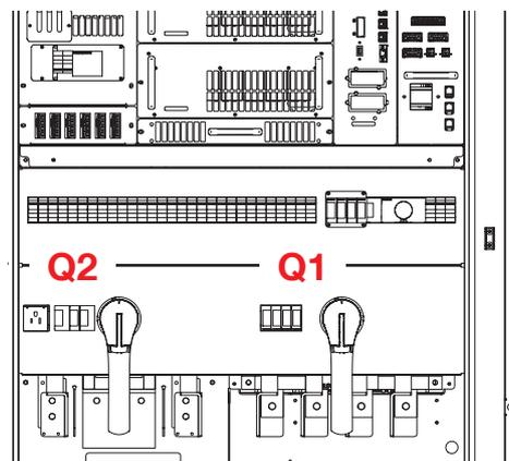
Figure 75. Location of the AC and DC switches (Q1 and Q2) in the C-Cab
