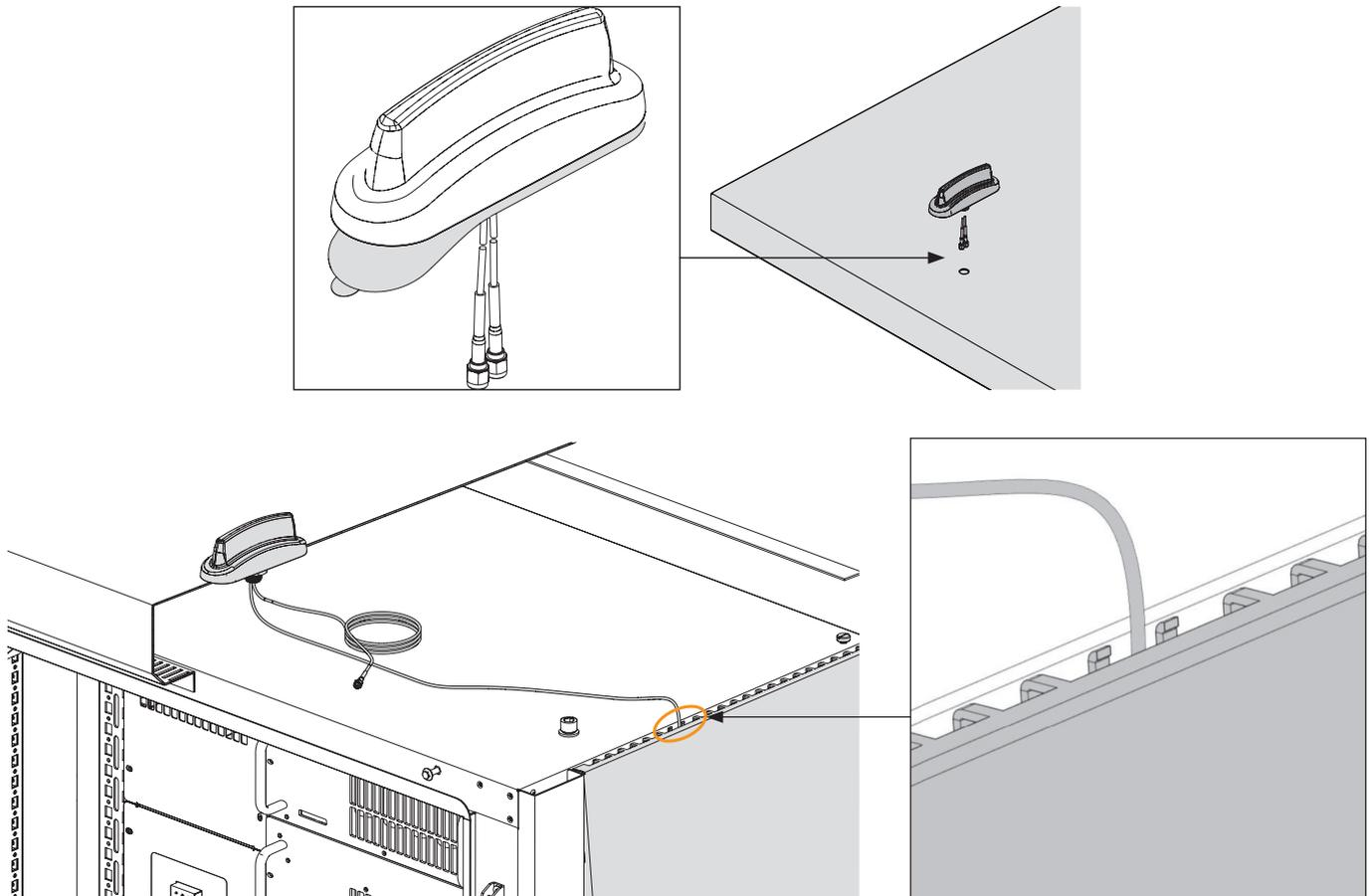
Figure 66. Antenna installation on the C-Cab
