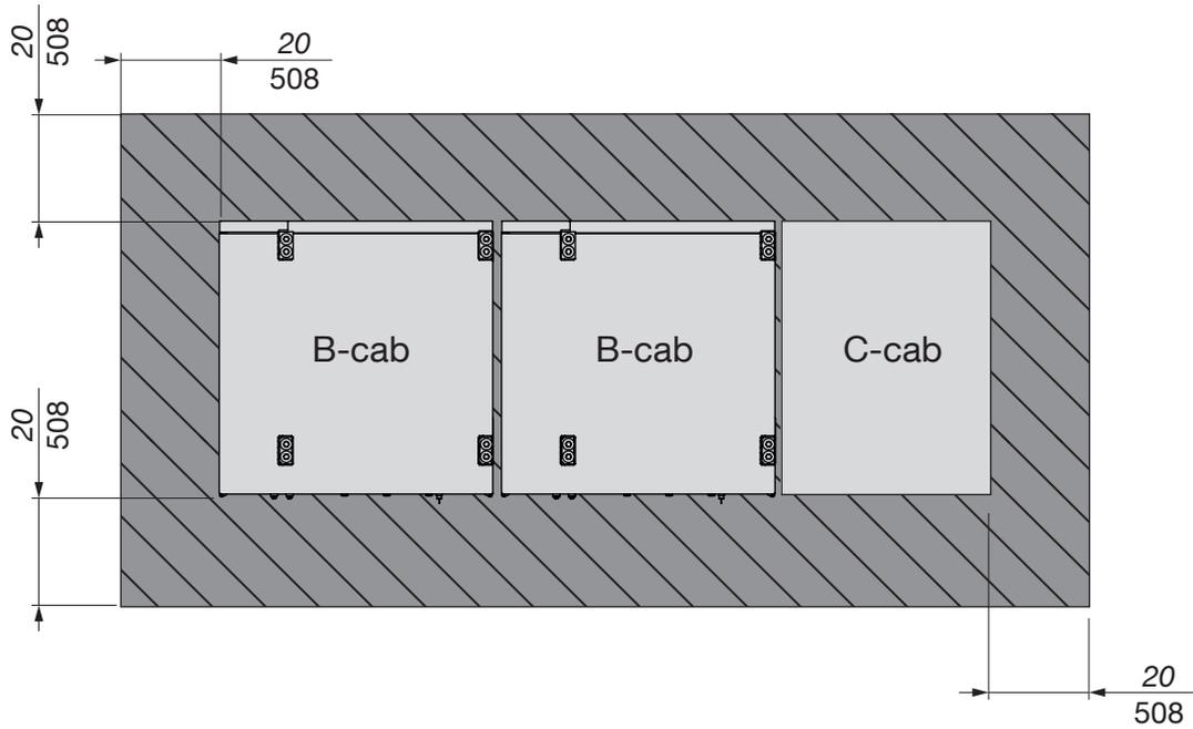
Figure 24. Concrete space around the equipment
