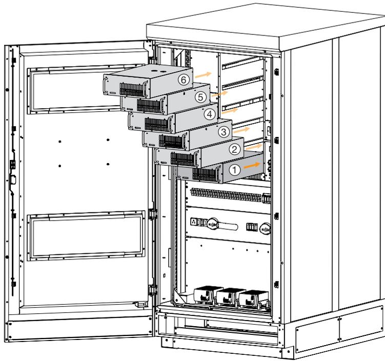
Figure 78. Order of insertion of the modules
