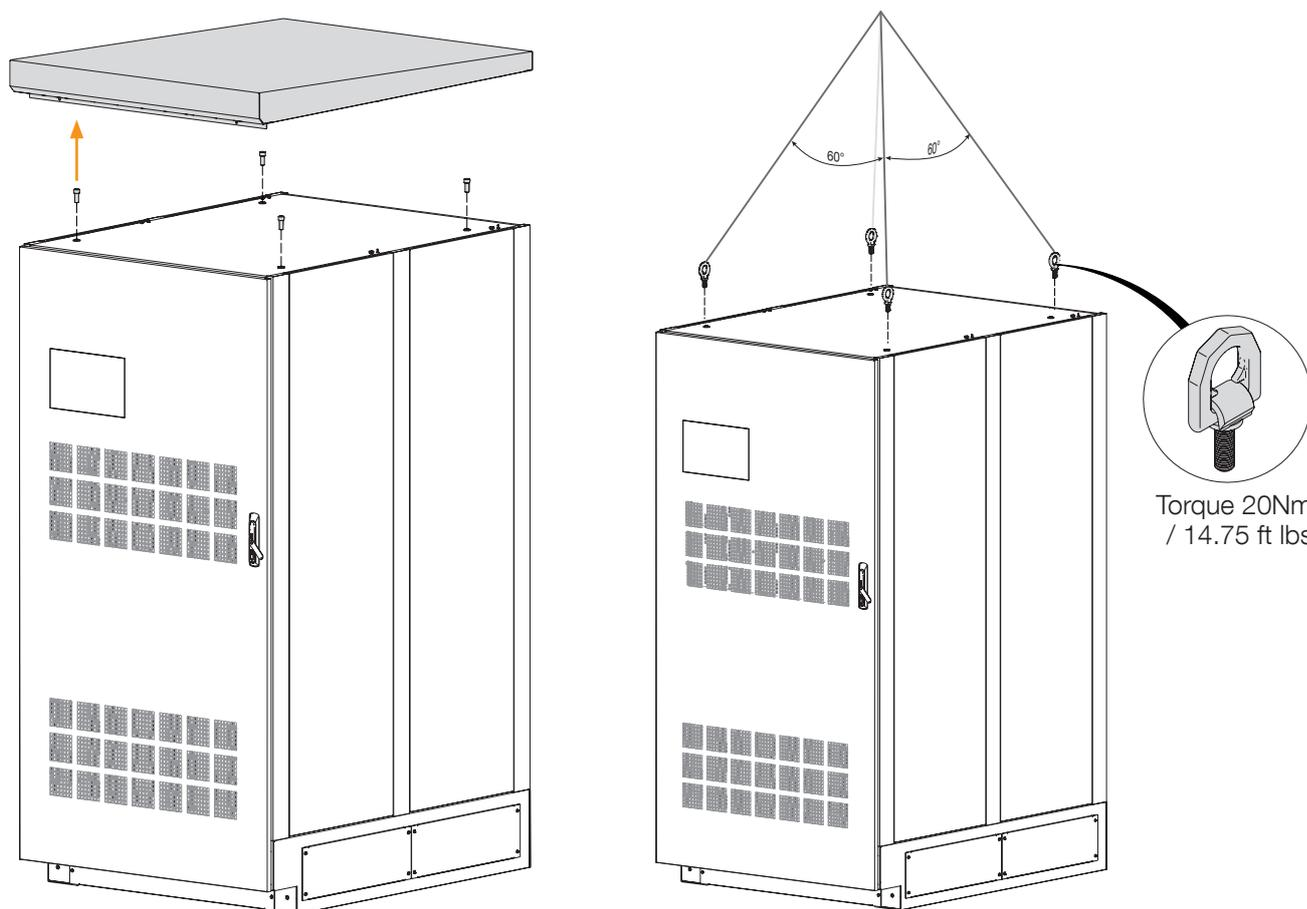
Figure 21. Lifting lugs on top of the C-Cab
