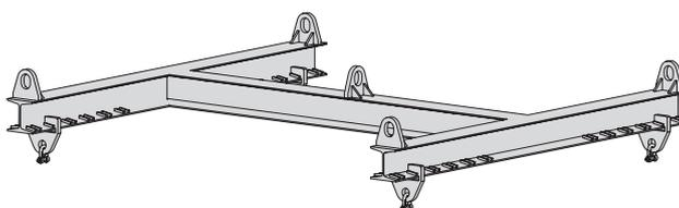
Figure 22. Vertical load spreader
