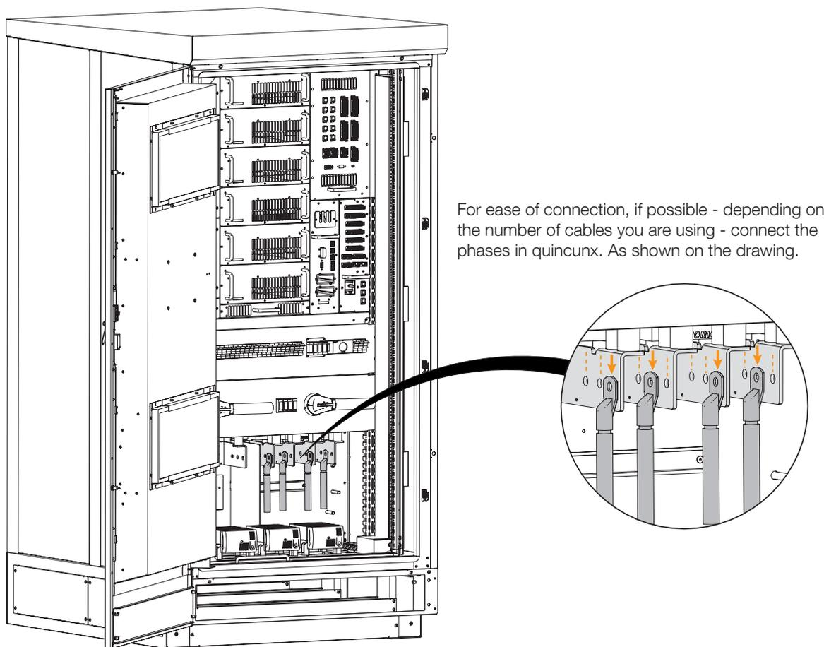
For ease of connection, if possible - depending on the number of cables you are using - connect the phases in quincunx. As shown on the drawing.
