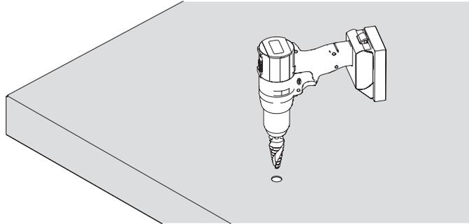
Figure 65. Hole drilling in the roof
