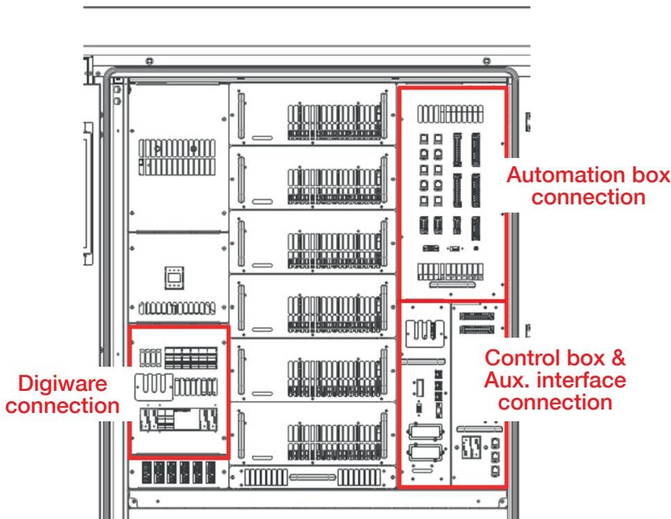
Figure 56. Location of the communication and signal connections in the C-Cab
