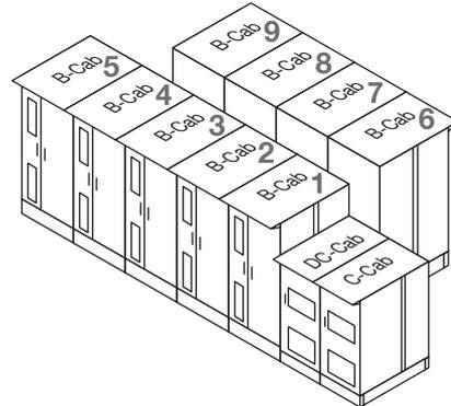
Figure 27. Back-to-back installation
