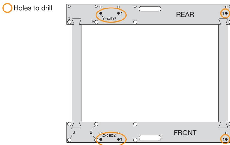
Figure 34. Holes to drill for 1 C-Cab + 1 C-Cab ext. installation
