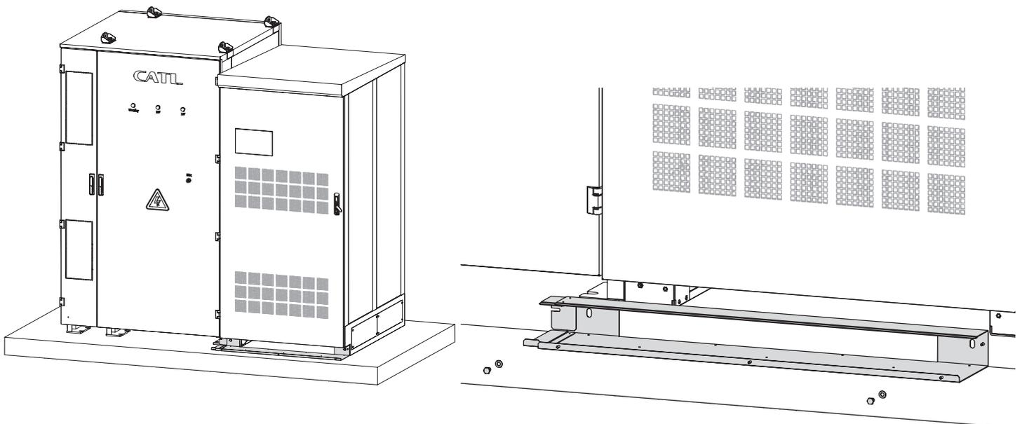
Figure 38. Installation of the back part of the C-Cab connection kit
