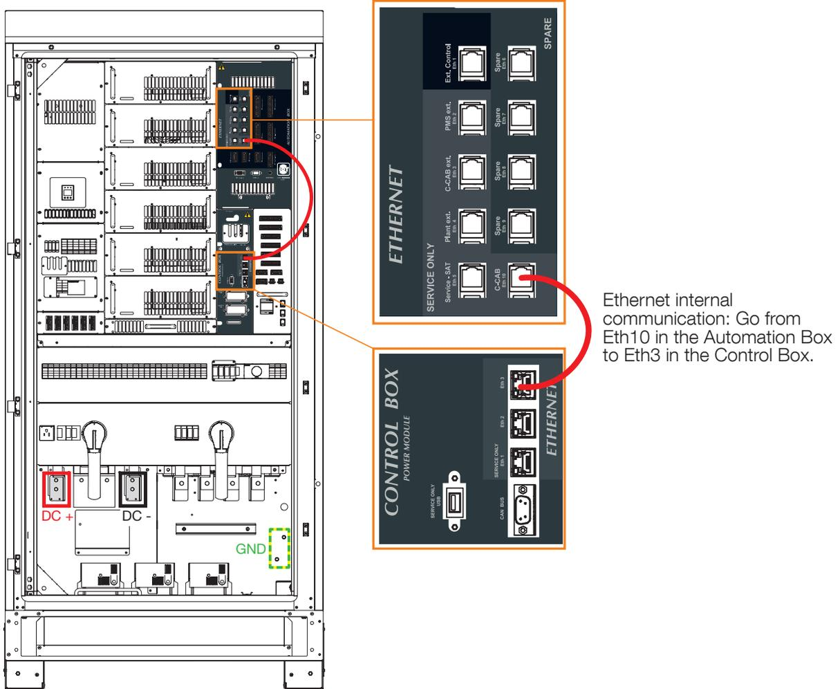
Figure 57. Connection of the communication with the control box
