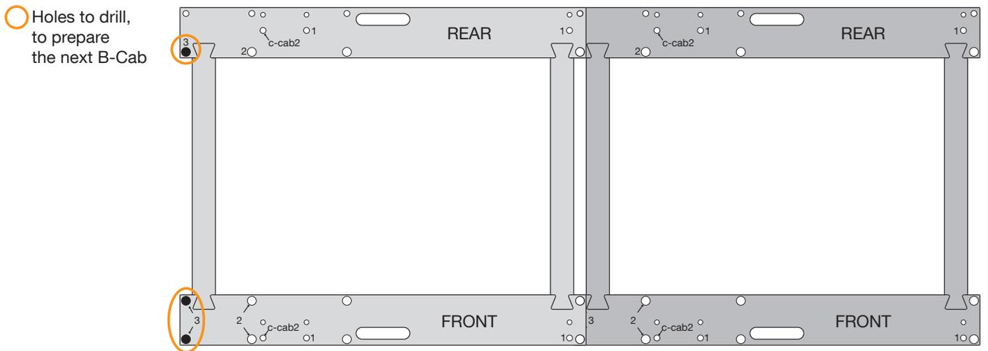
Figure 33. Holes to drill to prepare next B-cab installation
