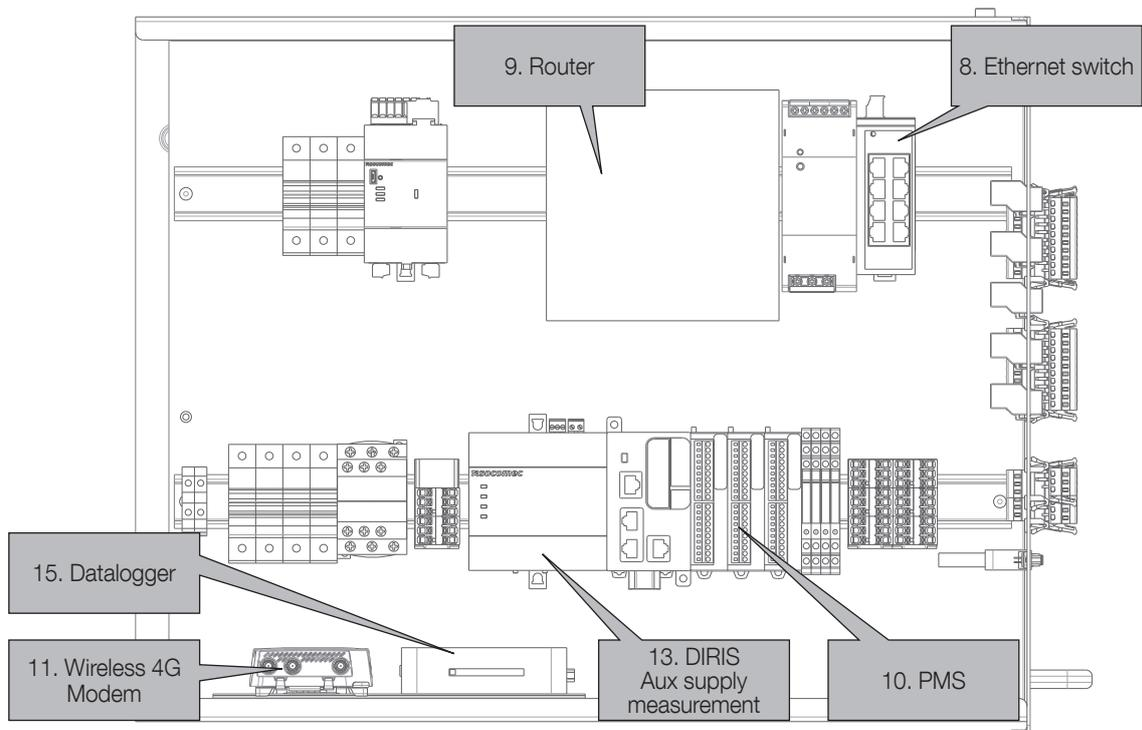
Figure 07. Detailed view of the Automation box
