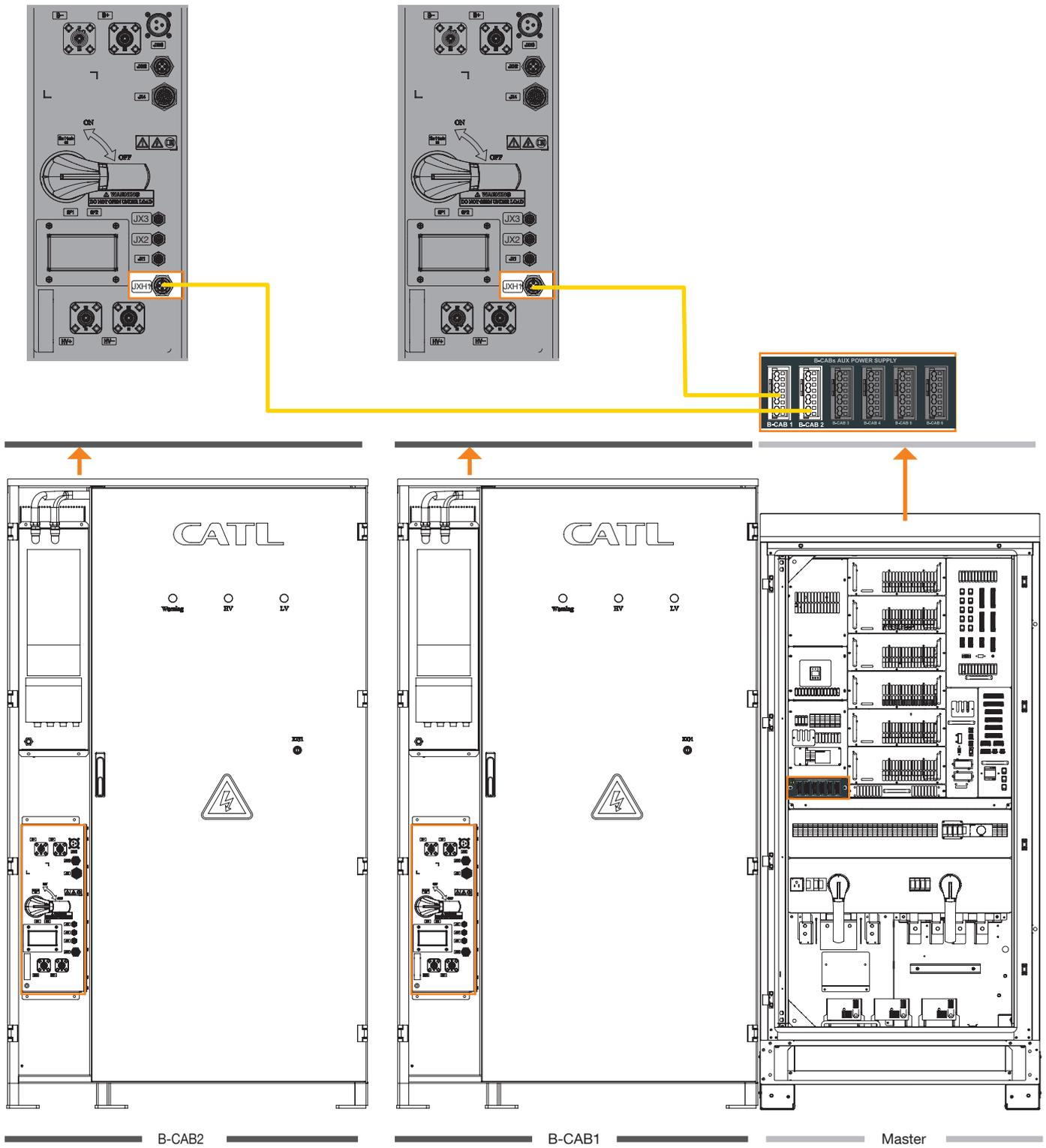
Figure 54. Connection of the B-Cabs aux power supply from the C-Cab
