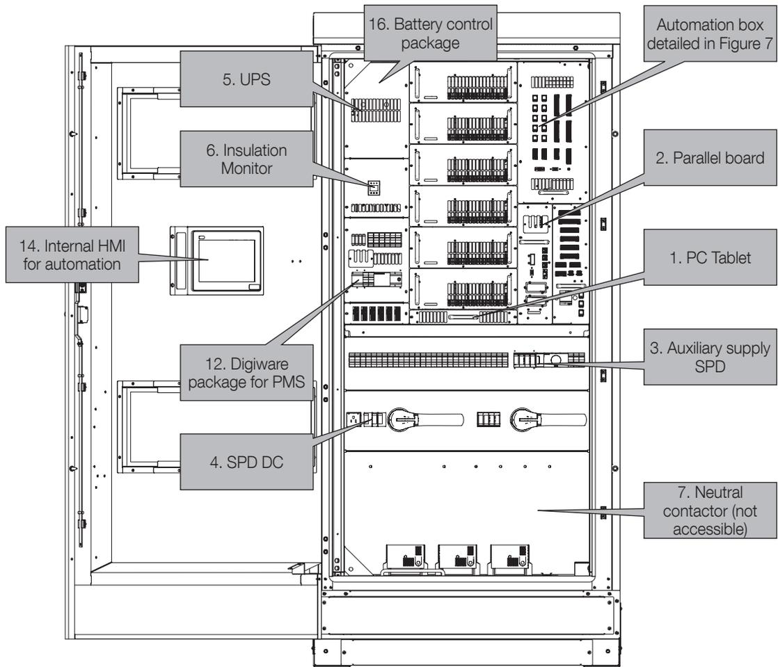
Figure 06. View of the dedicated components inside the C-Cab
