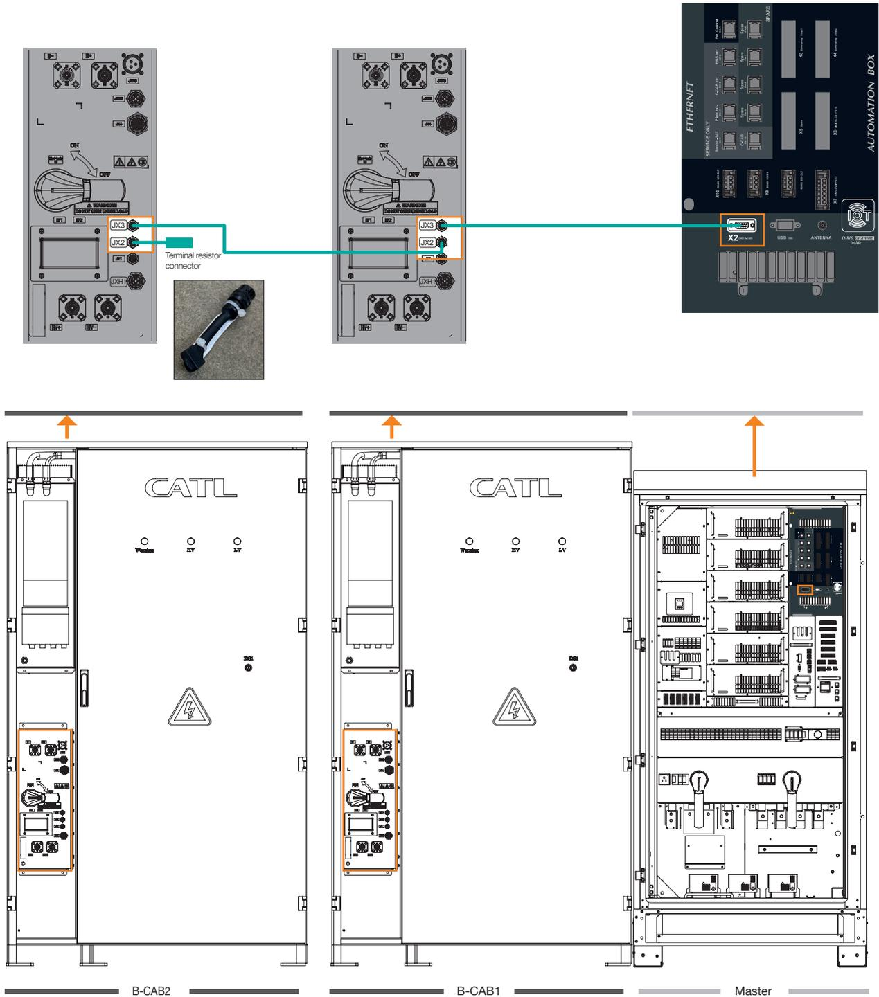
Figure 58. Connection of the communication between B-Cabs and C-Cab
