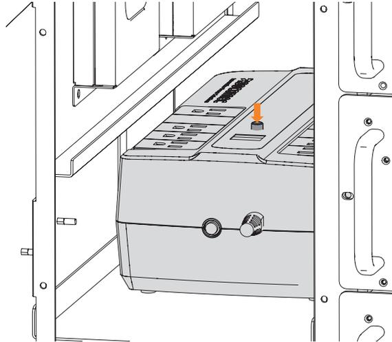
Figure 73. Location of the power button of the UPS
