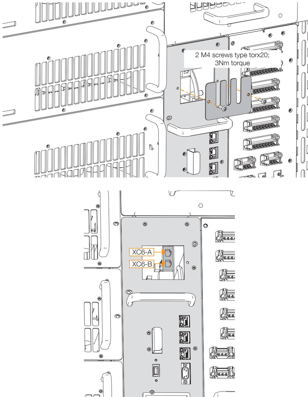
Figure 60. Location of the RJ cables for C-Cabs Master-Extension paralleling
