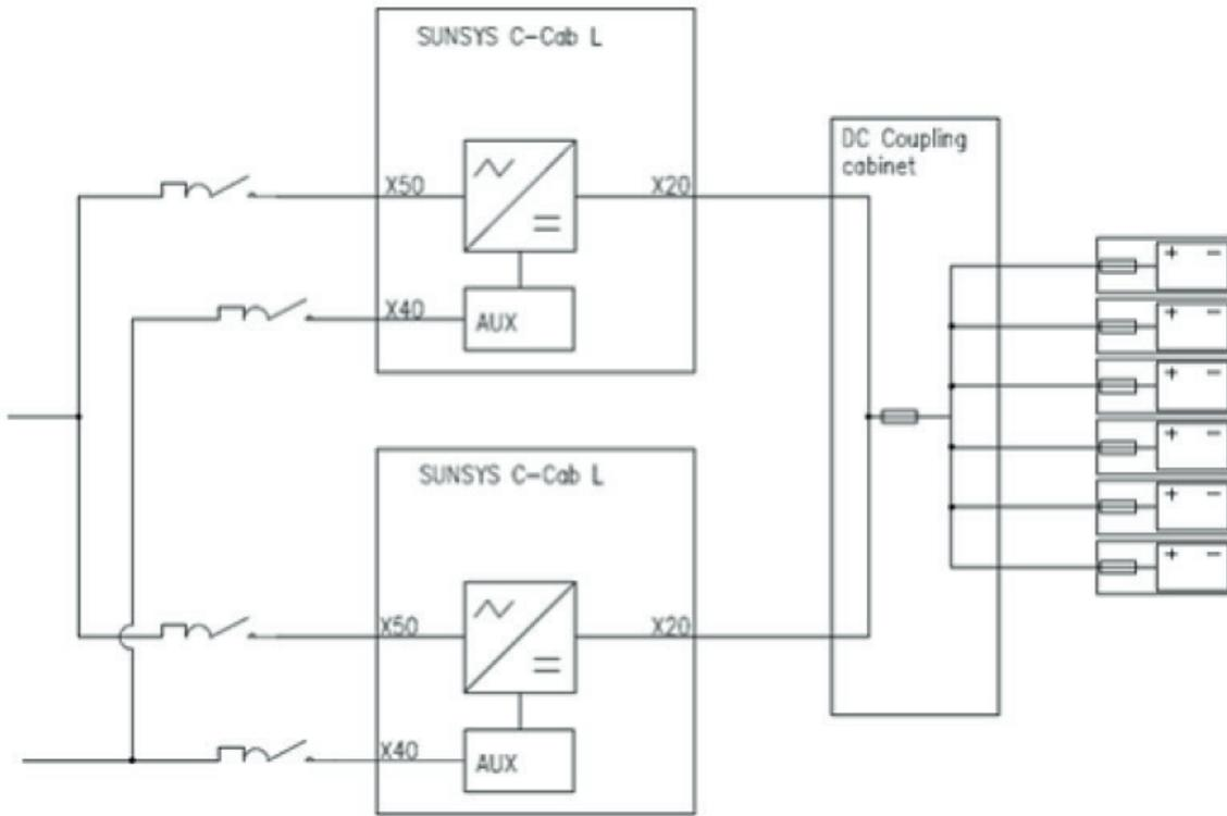
Protection of 2 C-Cabs with common AC protection (allowed) without DC-Cab
