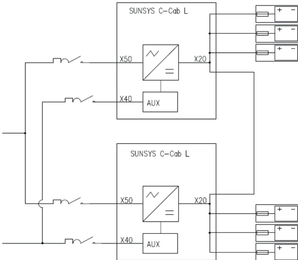
Protection of 2 C-Cabs with 2 separated AC protections (suggested) with DC-Cab
