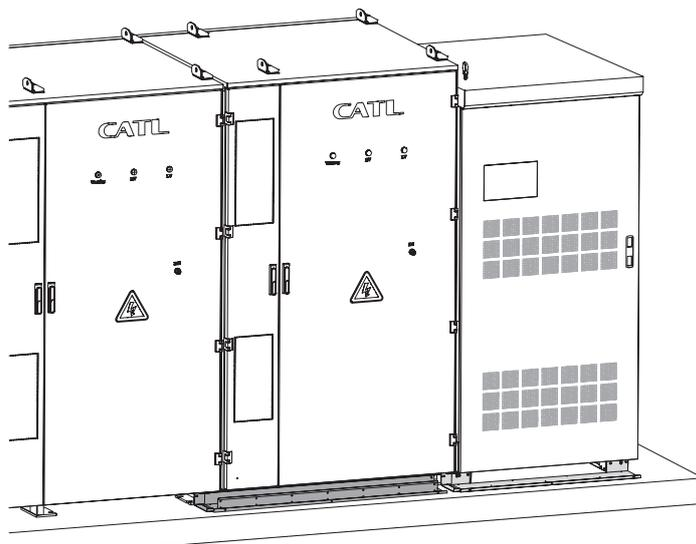
Figure 41. Installation of the B-Cab back part connection kit
