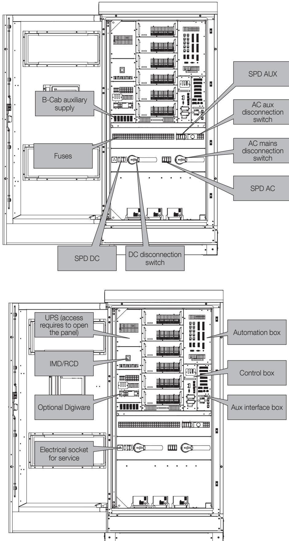
Figure 08. View of the devices accessible from the front of the C-Cab
