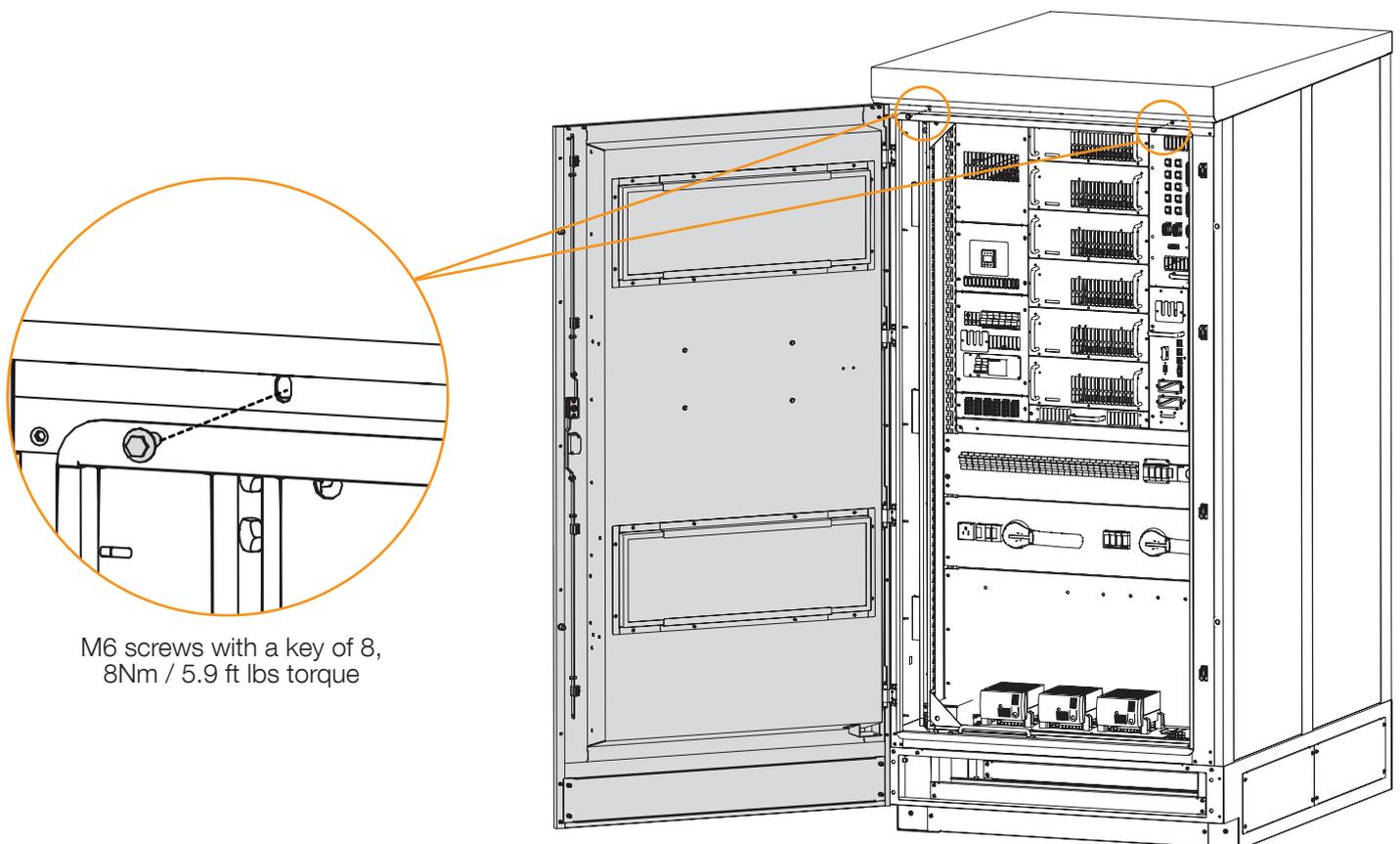
Figure 20. C-Cabs front top screws
