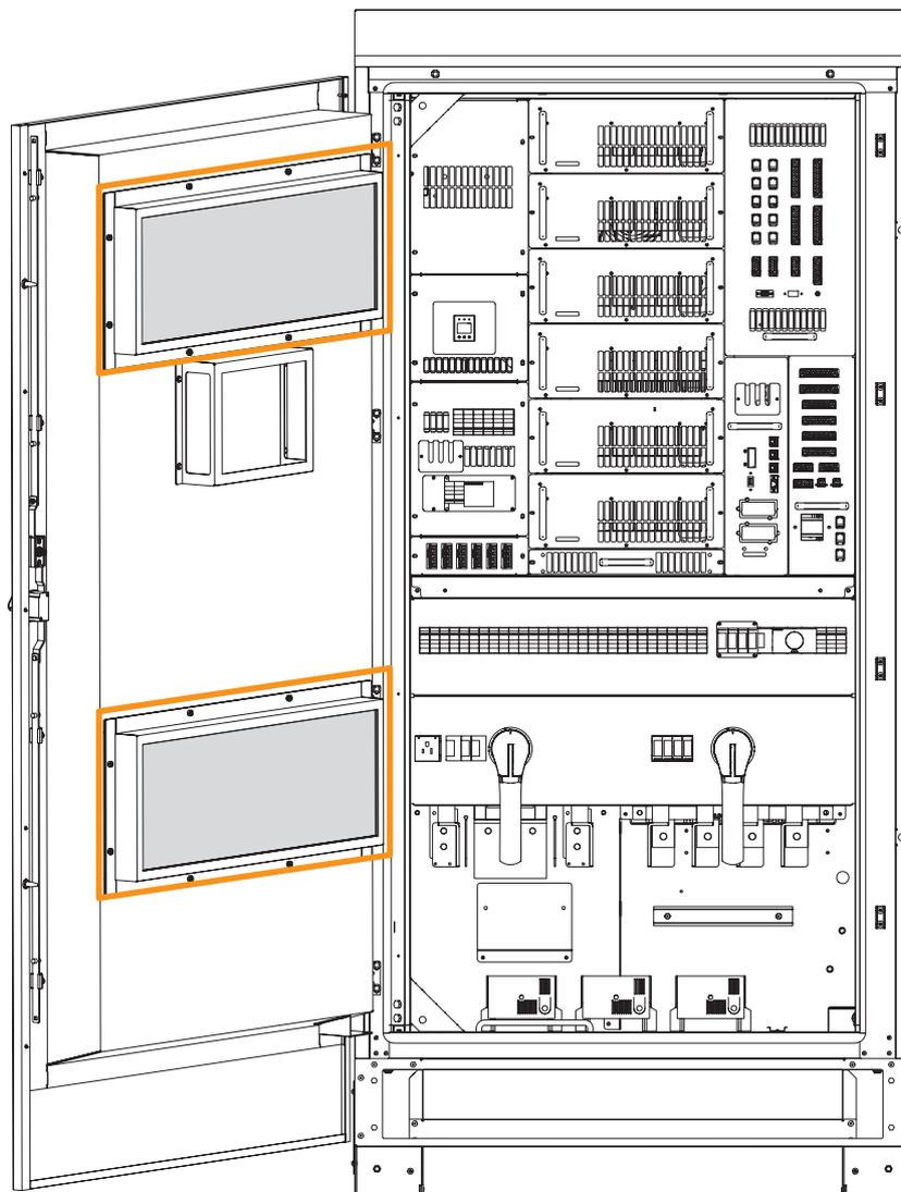
Figure 79. Location of the C-Cab air filters
