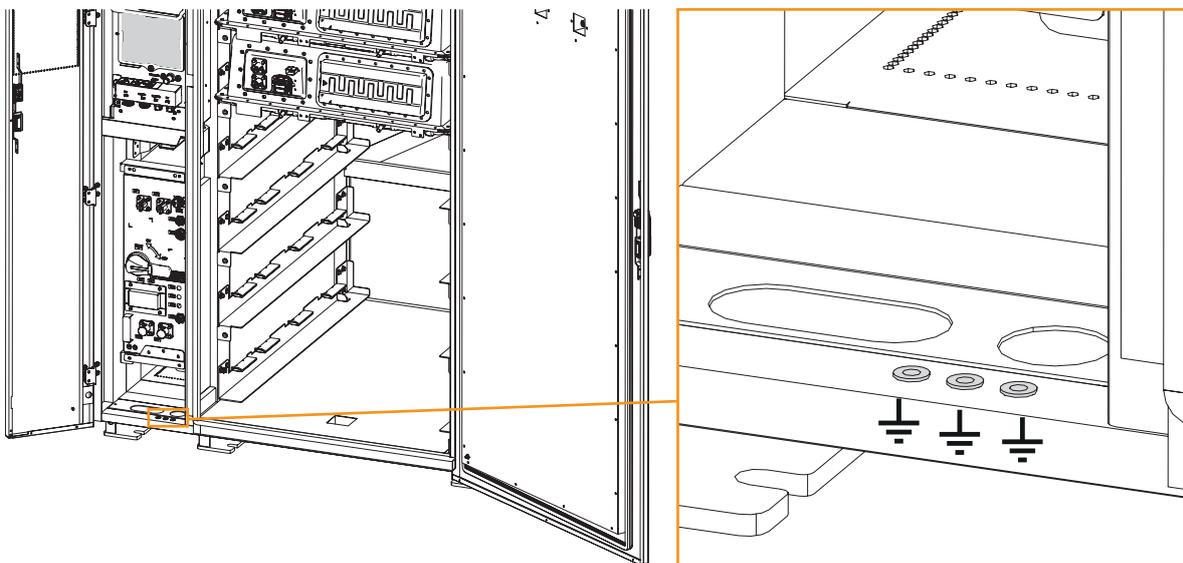
Figure 51. Battery cabinet ground terminal
