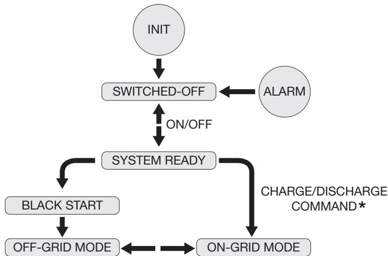
Figure 09. Modes of operation of SUNSYS HES L
