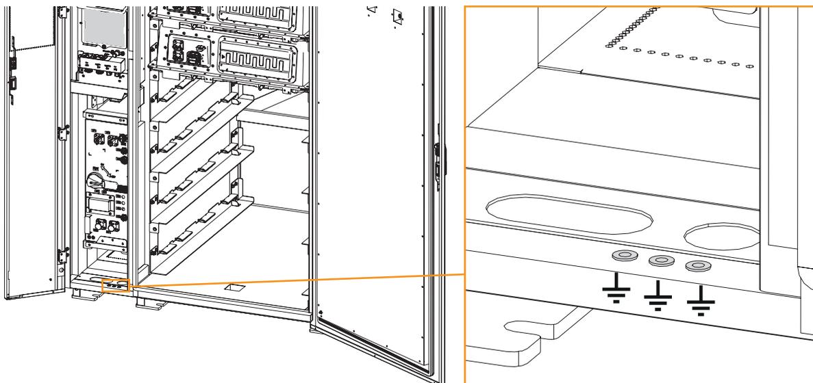
Figure 48. Battery cabinet ground terminal
