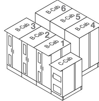
Figure 27. Back-to-back installation
