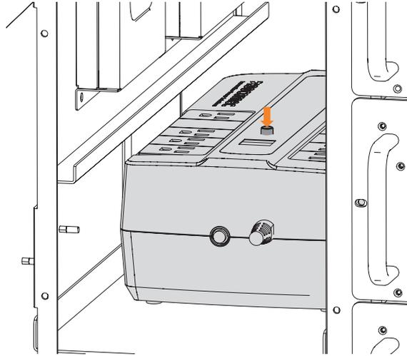
Figure 65. Location of the power button of the UPS
