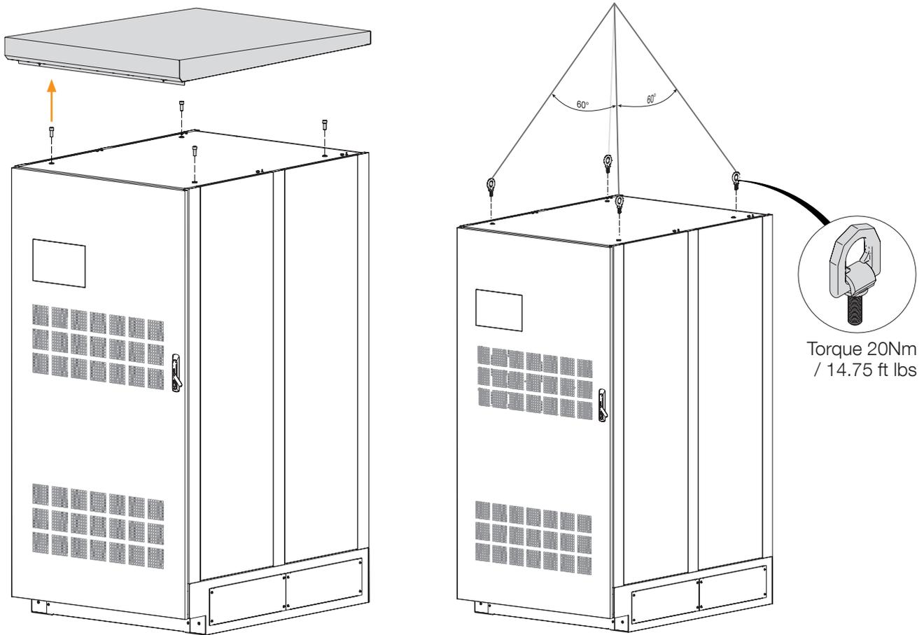
Figure 21. Lifting lugs on top of the C-Cab
