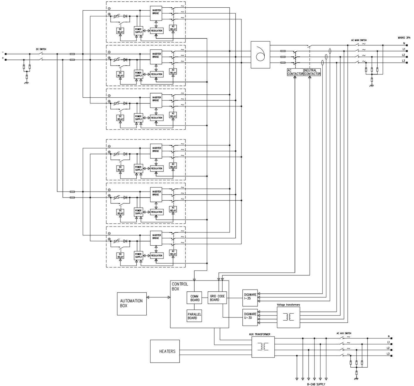
Figure 08. Example of C-Cab layout with autotransformer and options installed
