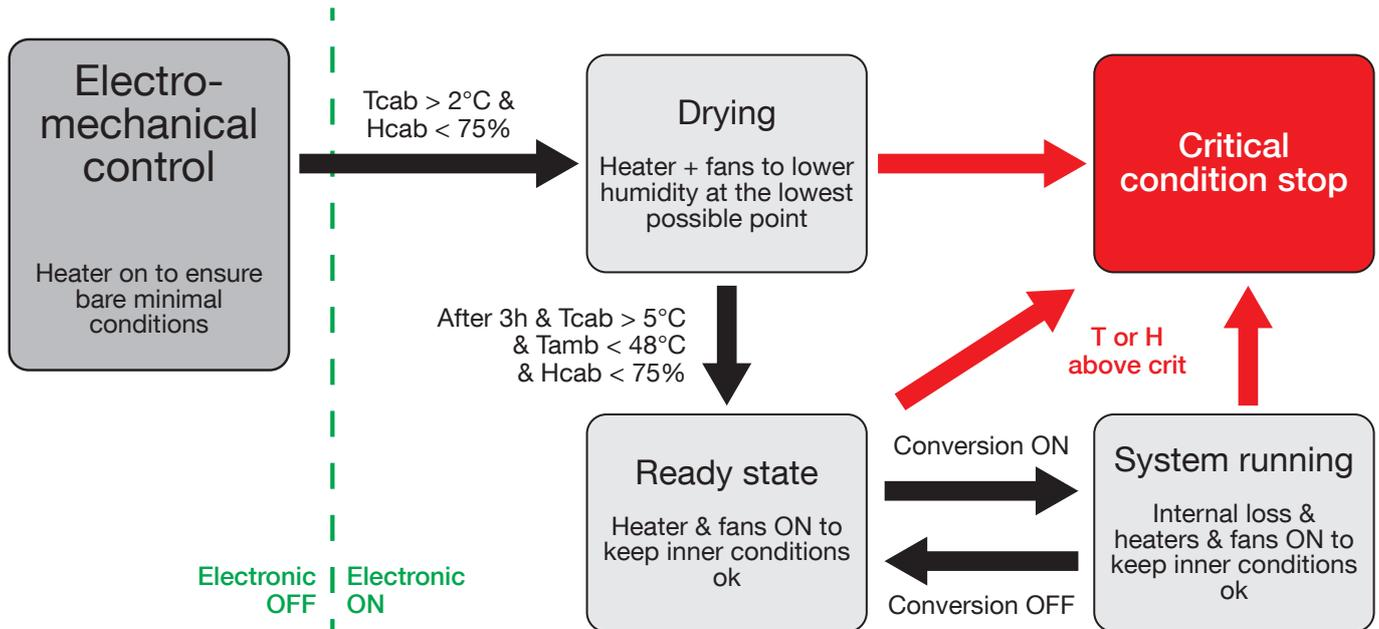
Figure 12. Environmental logic diagram
