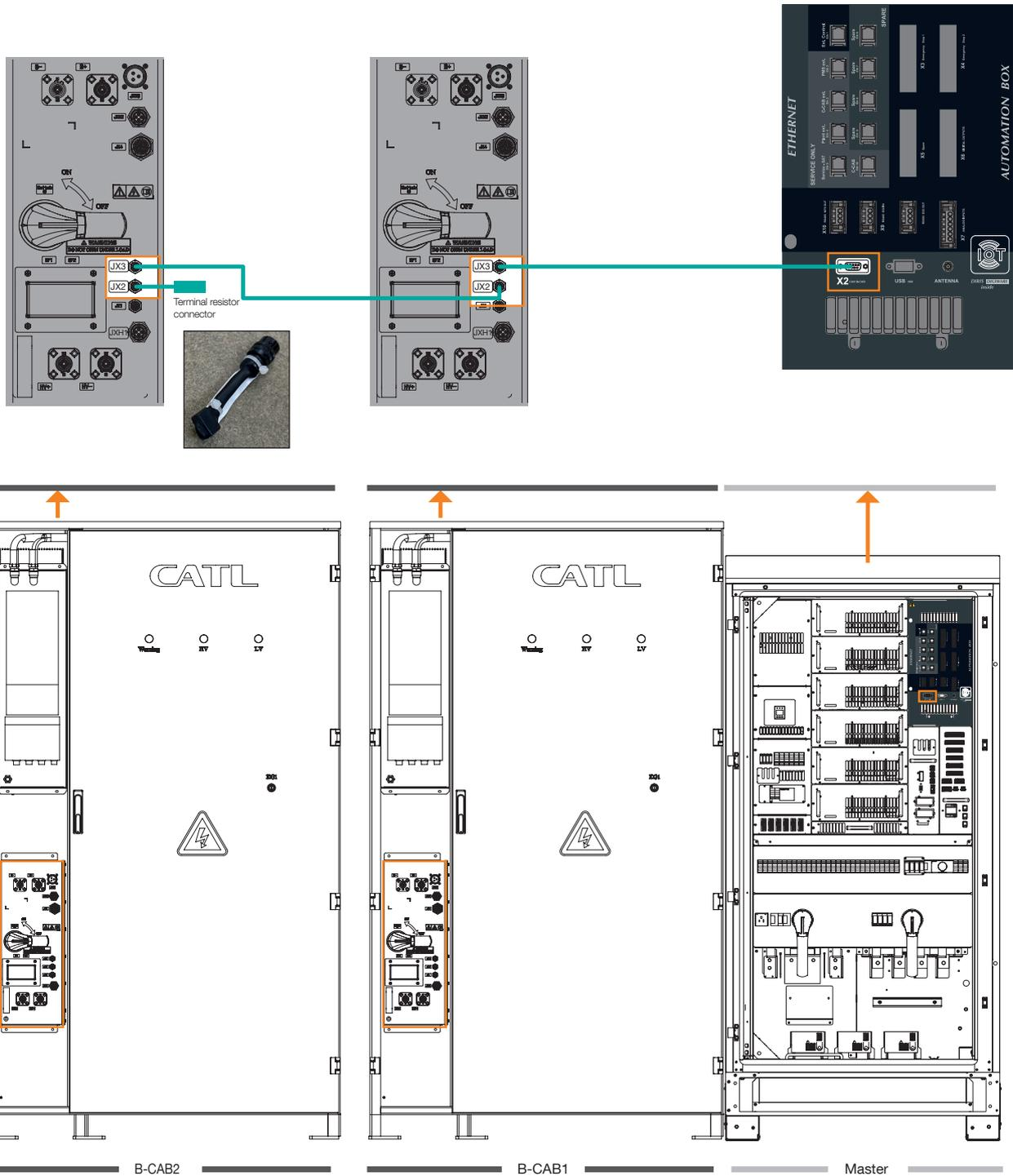
Figure 55. Connection of the communication between B-Cabs and C-Cab
