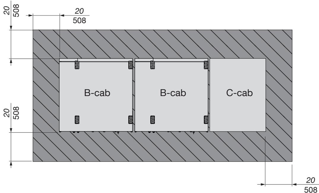
Figure 24. Concrete space around the equipment
