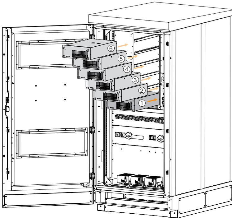
Figure 70. Order of insertion of the modules
