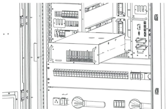
Figure 69. Insertion of the power module
