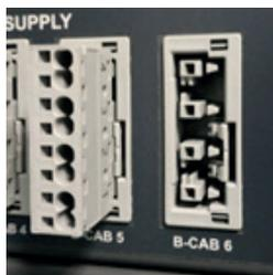
Figure 14. B-Cab aux supply connectors
