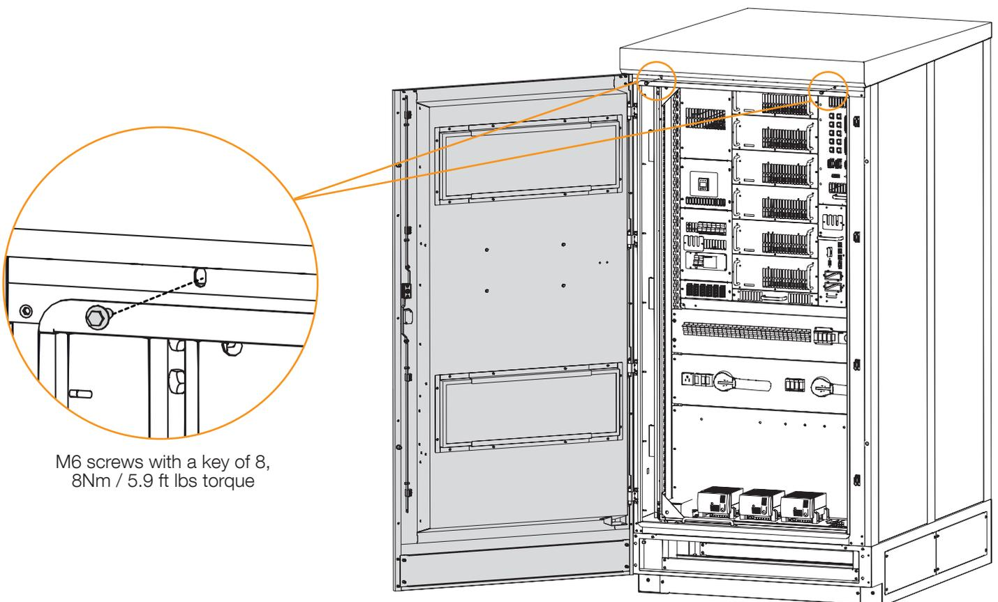
Figure 20. C-Cabs front top screws
