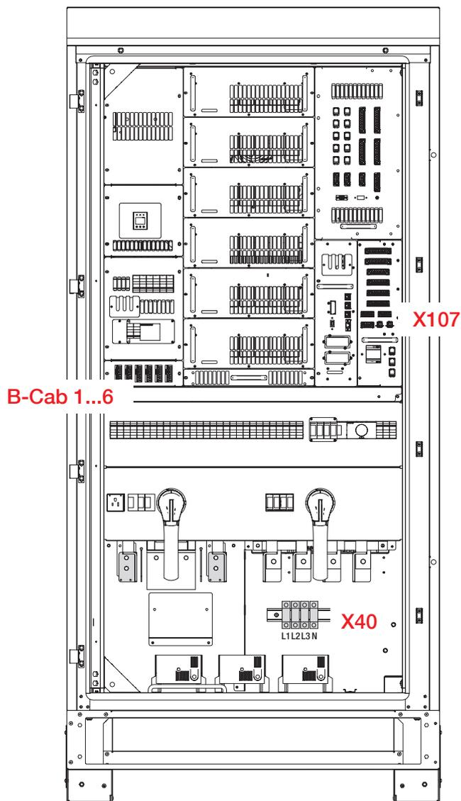
Figure 49. Location of the auxiliary connections in the C-Cab
