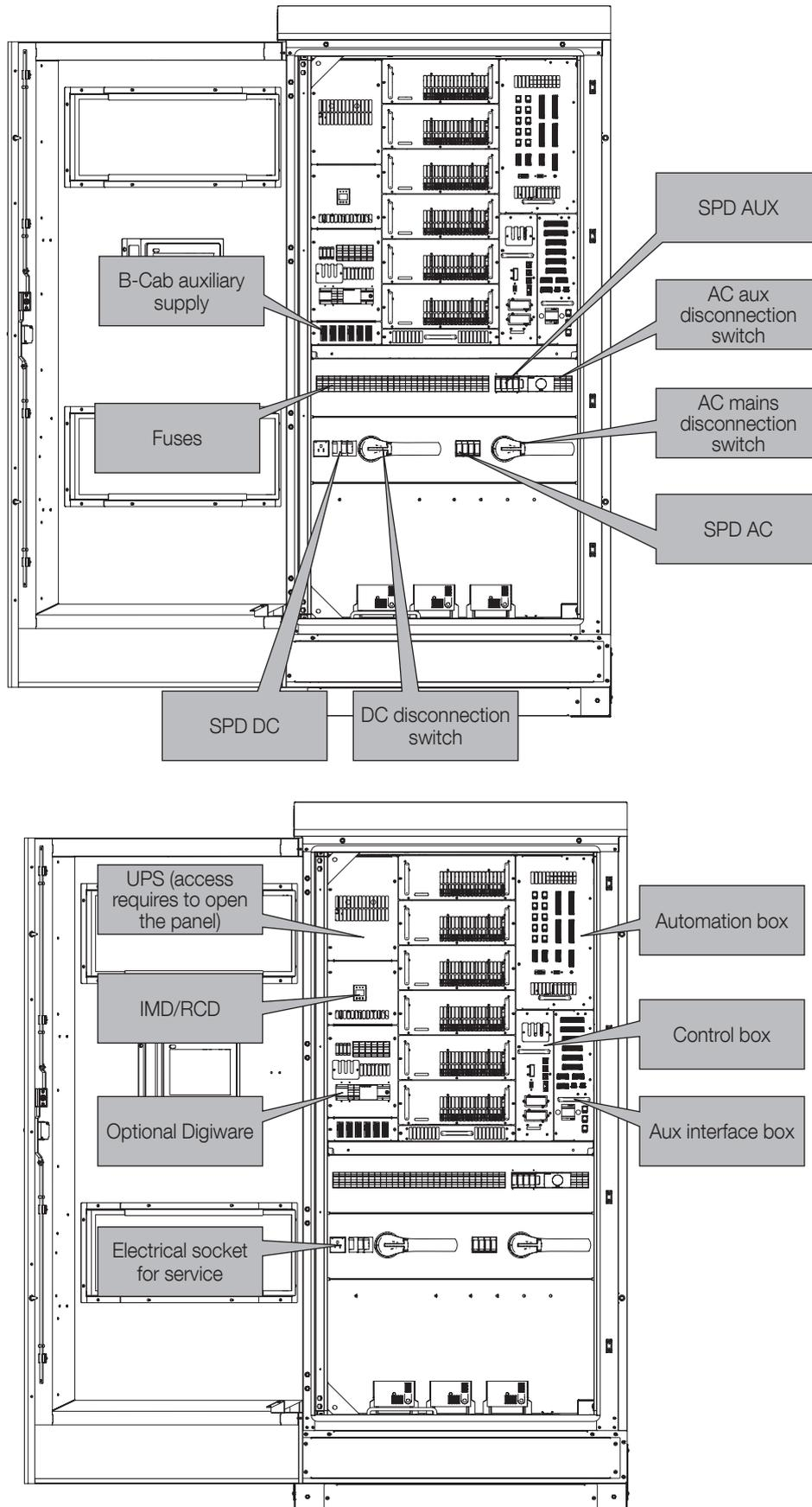
Figure 07. View of the devices accessible from the front of the C-Cab
