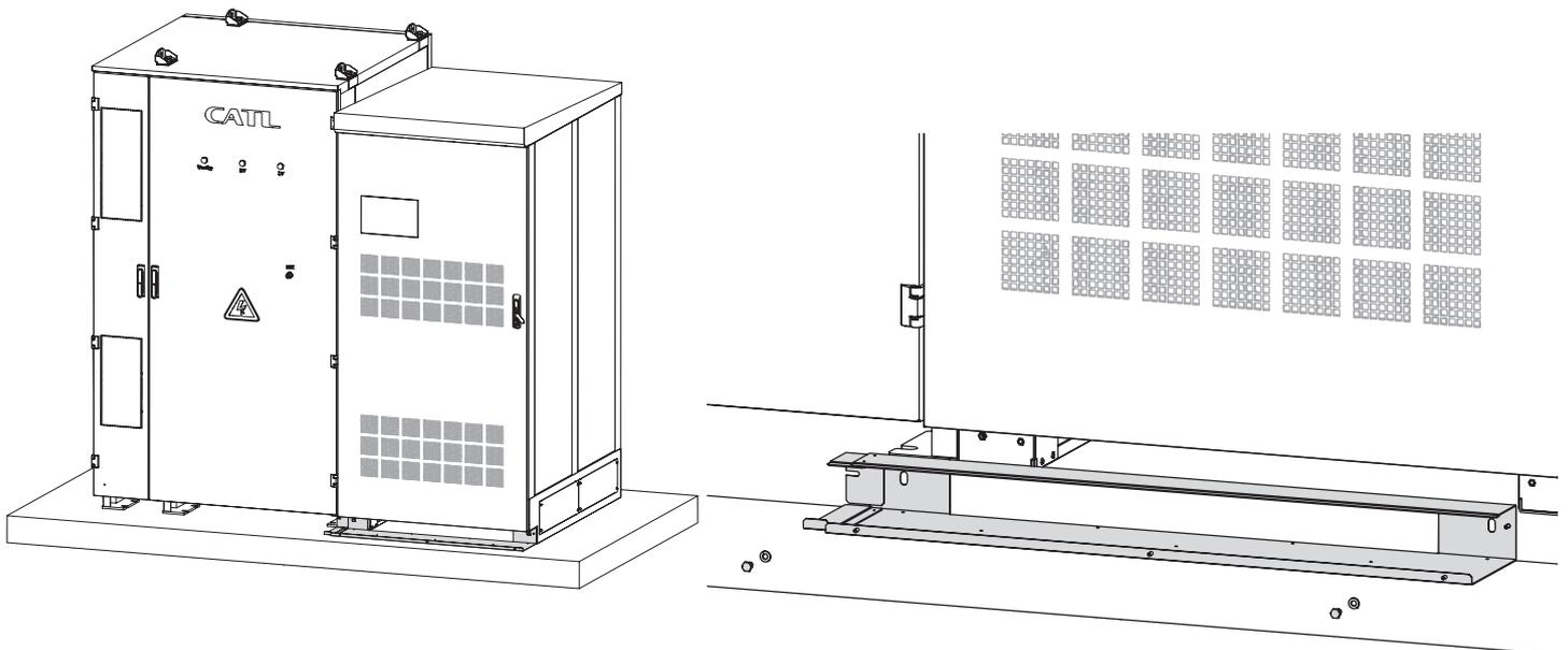
Figure 35. Installation of the back part of the C-Cab connection kit
