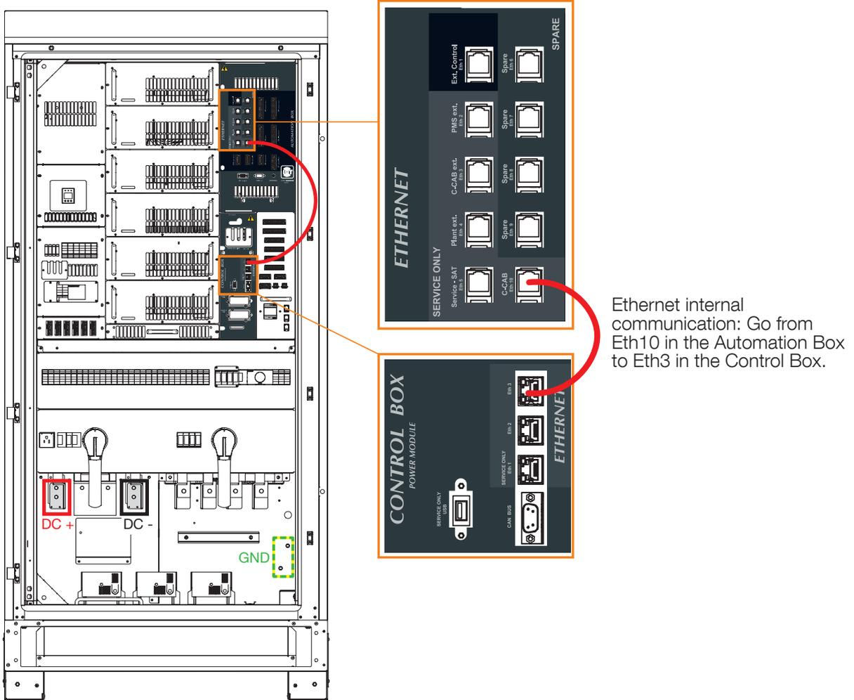
Figure 54. Connection of the communication with the control box
