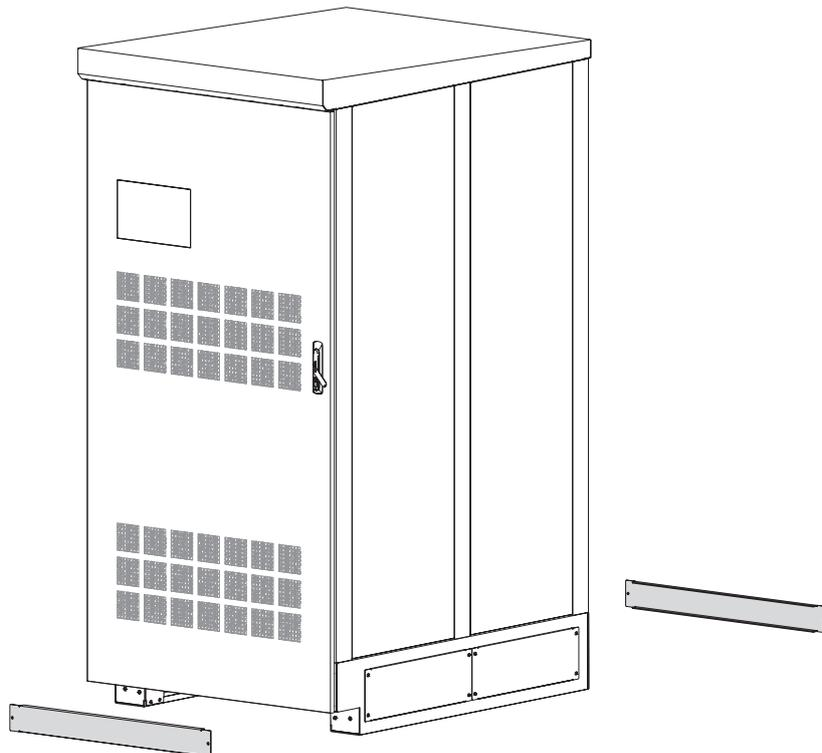
Figure 17. Panels to remove from the C-Cab
