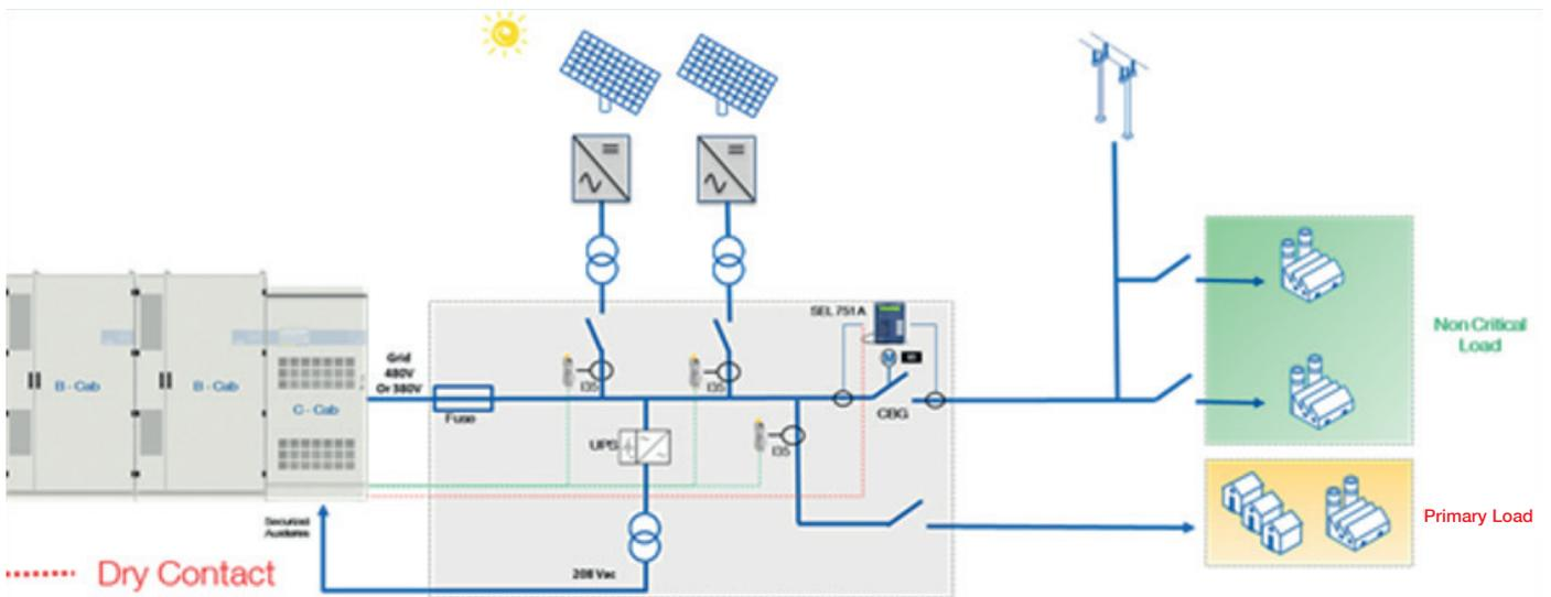
Figure 10. Architecture of the installation in case of operation with Islanding
