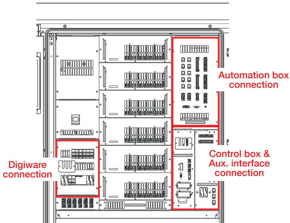
Figure 53. Location of the communication and signal connections in the C-Cab
