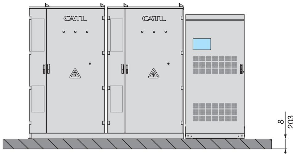
Figure 23. Concrete depth – SDS 2.5
