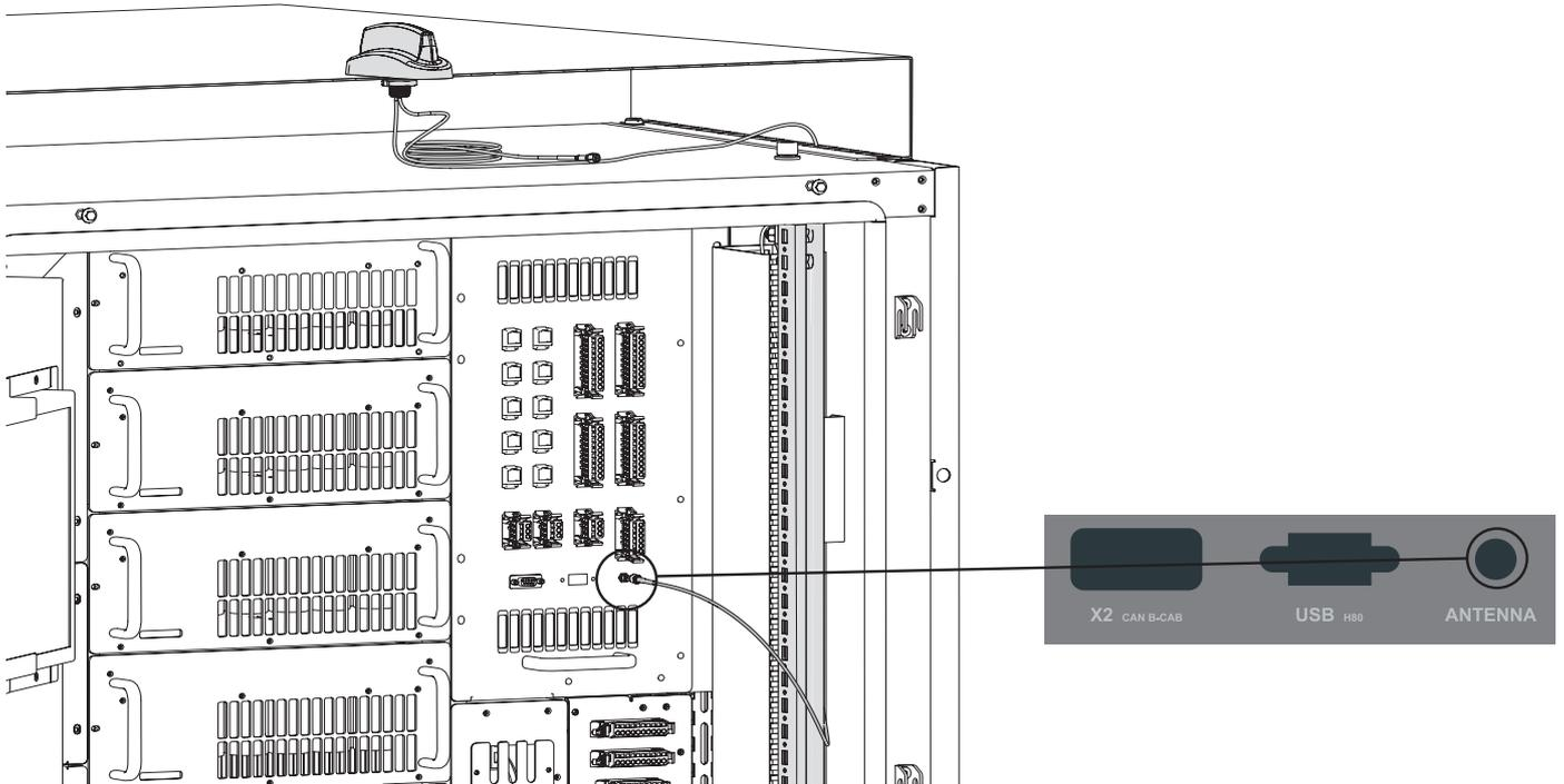
Figure 60. Connection of the antenna cable inside the C-Cab
