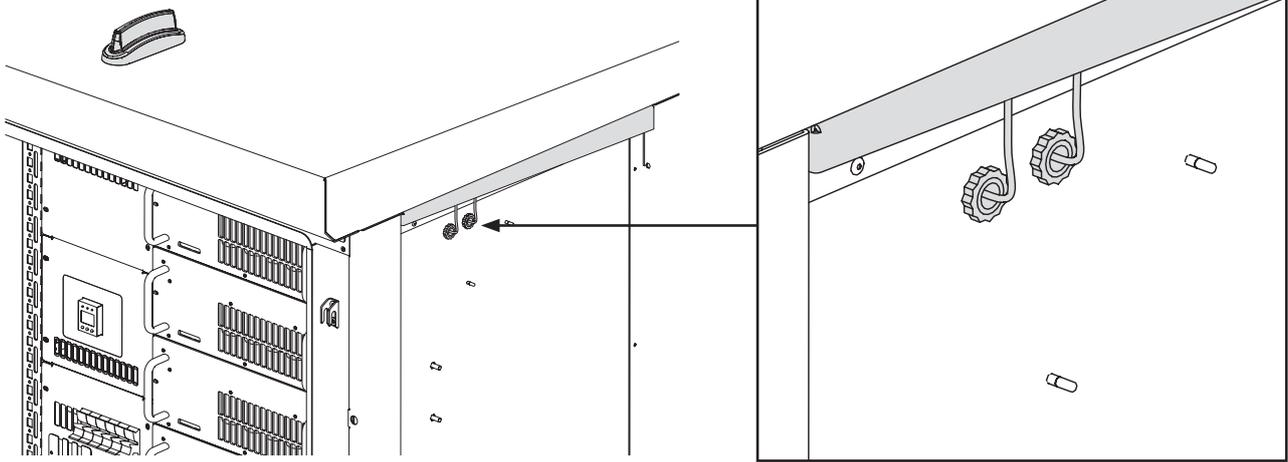
Figure 59. Cable direction from antenna to inside the C-Cab
