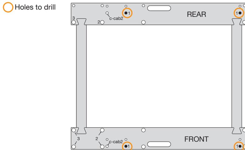
Figure 30. Holes to drill for 1 C-Cab installation
