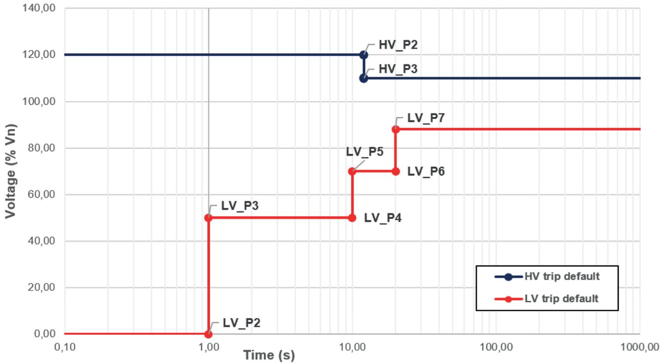
This voltage trip curves comply with the trip times as per IEEE 1547-2018 and IEEE 1547a-2020.
