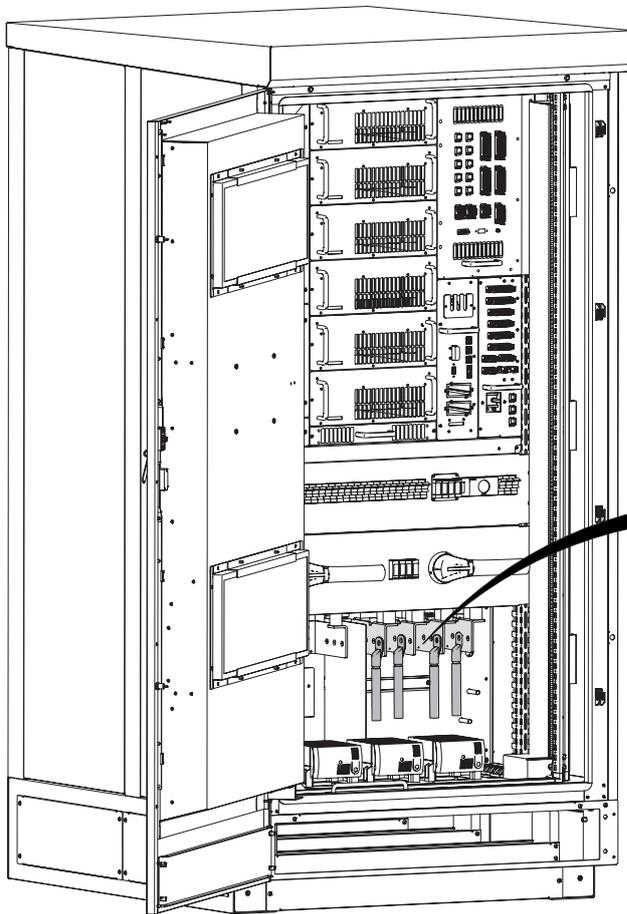
For ease of connection, if possible - depending on the number of cables you are using - connect the phases in quincunx. As shown on the drawing.
