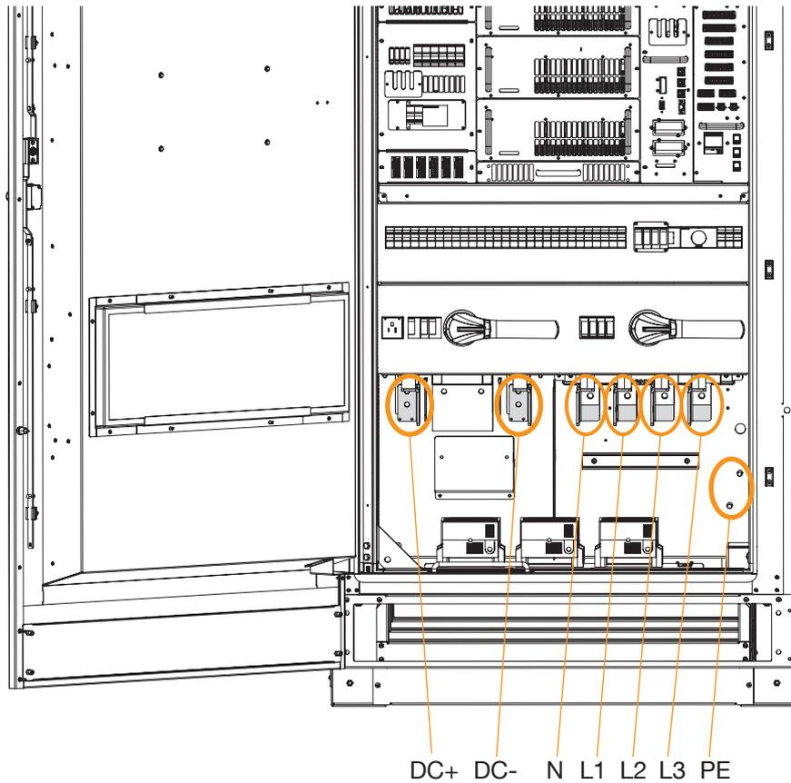
Figure 46. Power and ground connections
