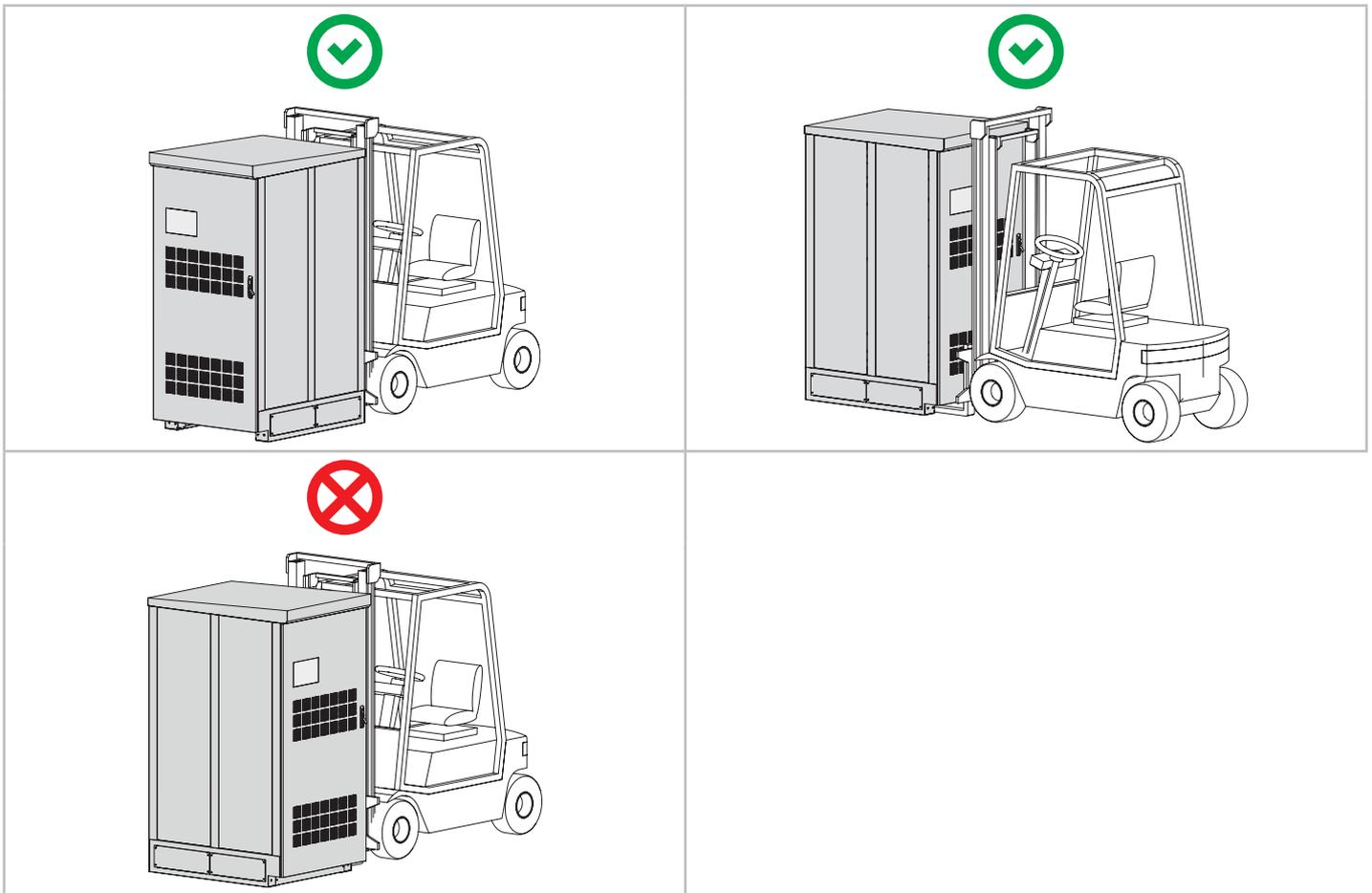
Figure 18. Handling of the unit using pallet truck with 1.30m long forks
