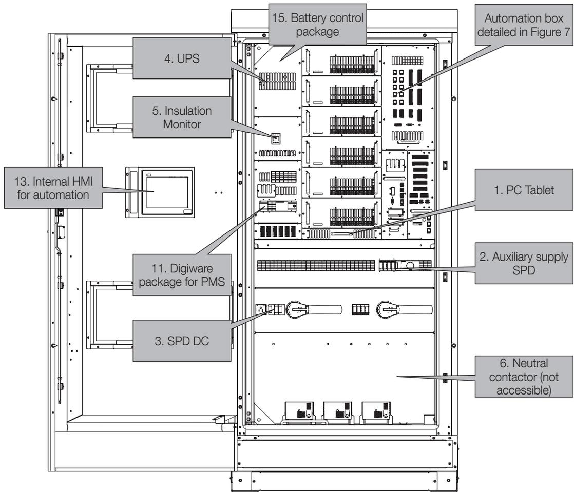
Figure 05. View of the dedicated components inside the C-Cab
