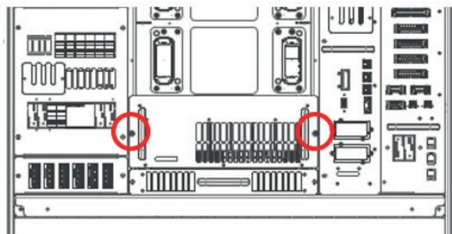
Figure 68. Power module screws location
