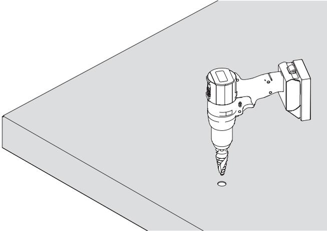
Figure 57. Hole drilling in the roof
