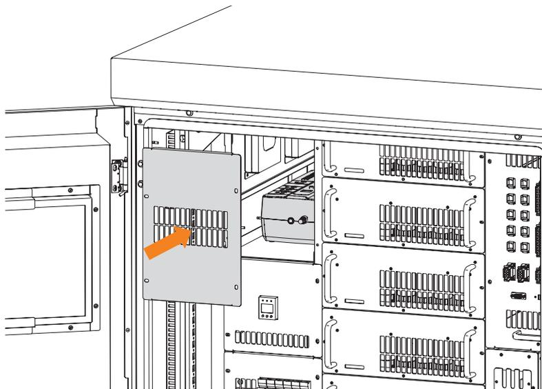
Figure 66. Reinstallation of the panel
