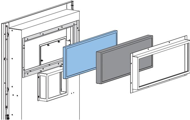
Figure 73. Installation of the air filter
