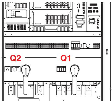
Figure 67. Location of the AC and DC switches (Q1 and Q2) in the C-Cab
