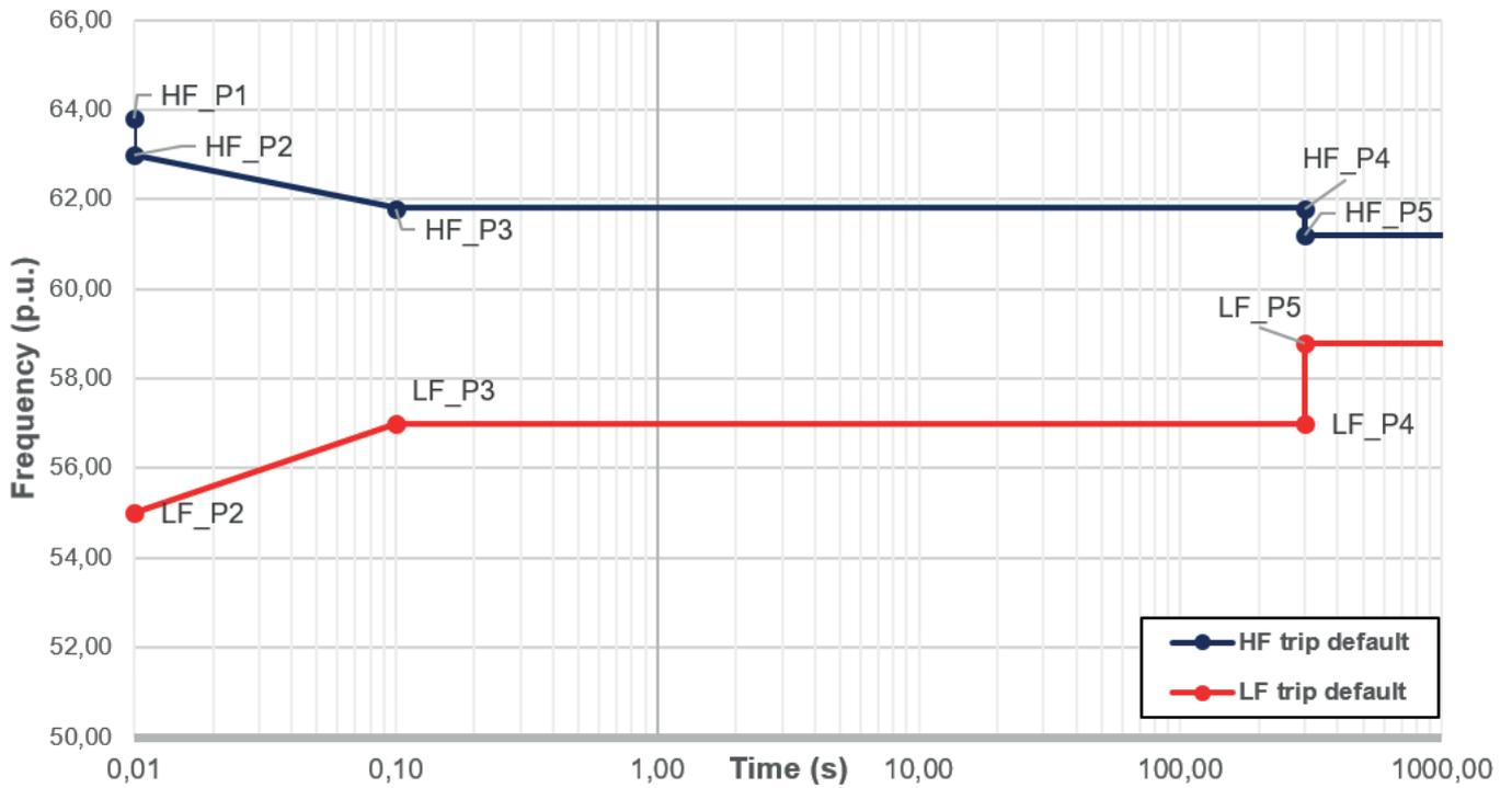
This frequency trip curves comply with the trip times as per IEEE 1547-2018 and IEEE 1547a-2020.
