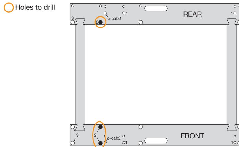
Figure 31. Holes to prepare B-Cab installation next to the C-Cab
