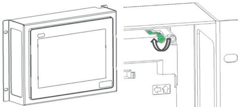
3. Mount the support with the HMI back on the door
