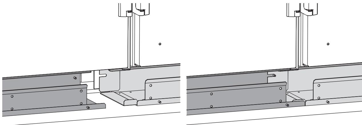
Figure 40. Connection of two B-Cab parts
