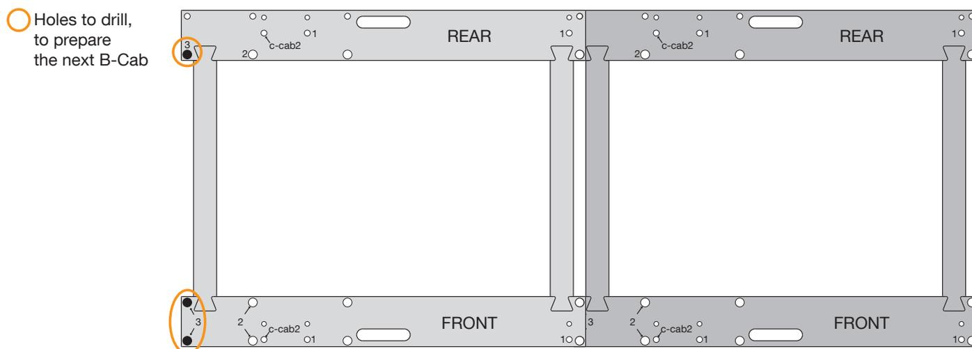
Figure 33. Holes to drill to prepare next B-cab installation
