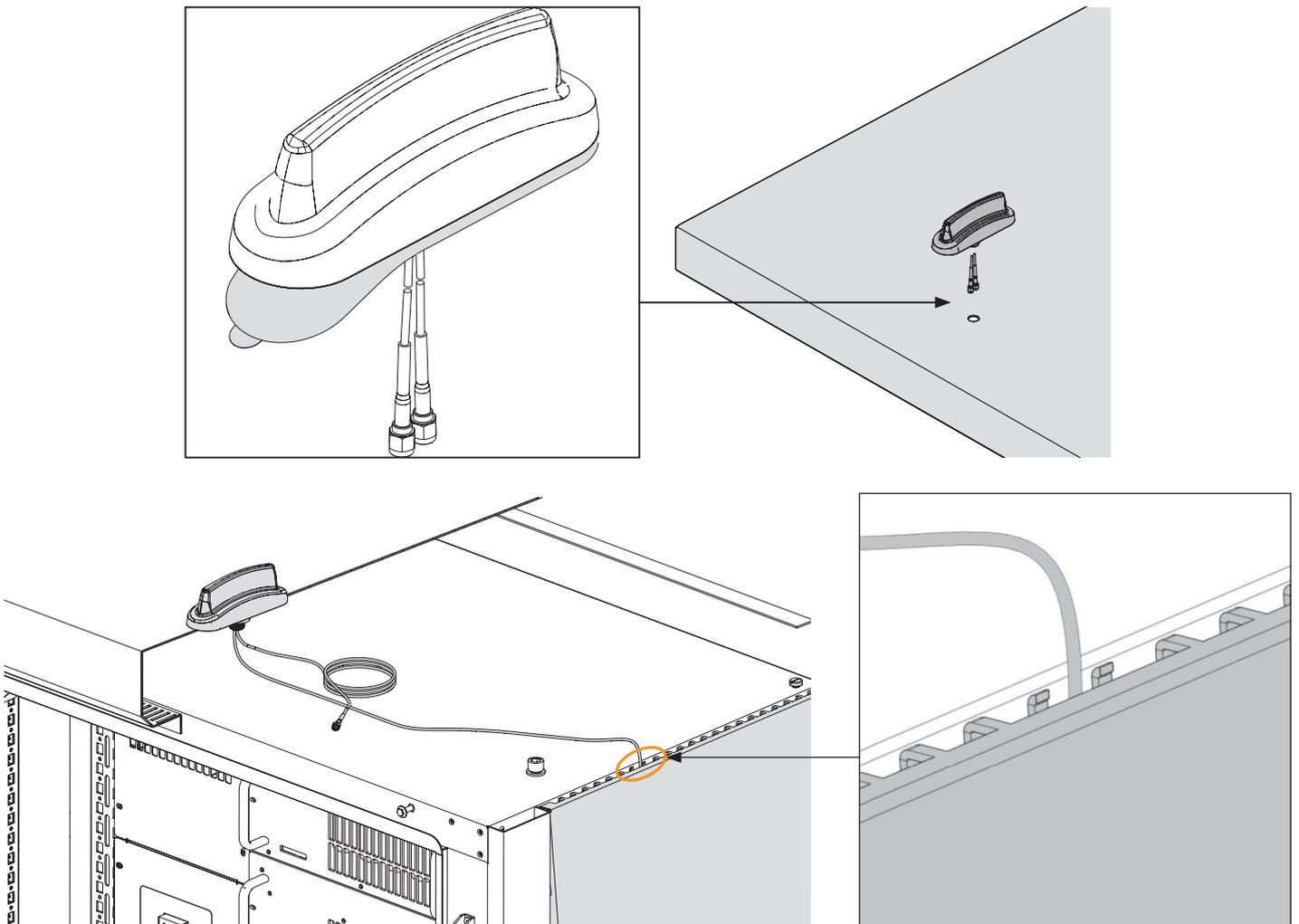
Figure 58. Antenna installation on the C-Cab
