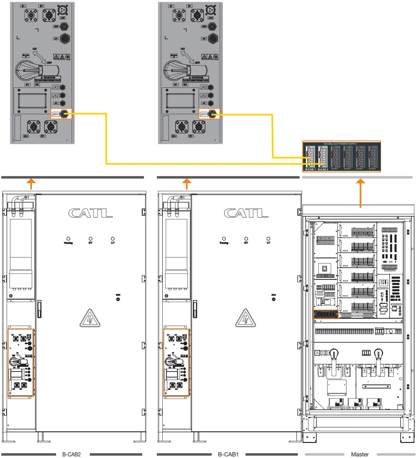
Figure 51. Connection of the B-Cabs aux power supply from the C-Cab
