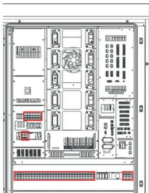
Figure 56. Location of the fuses inside the C-Cab
