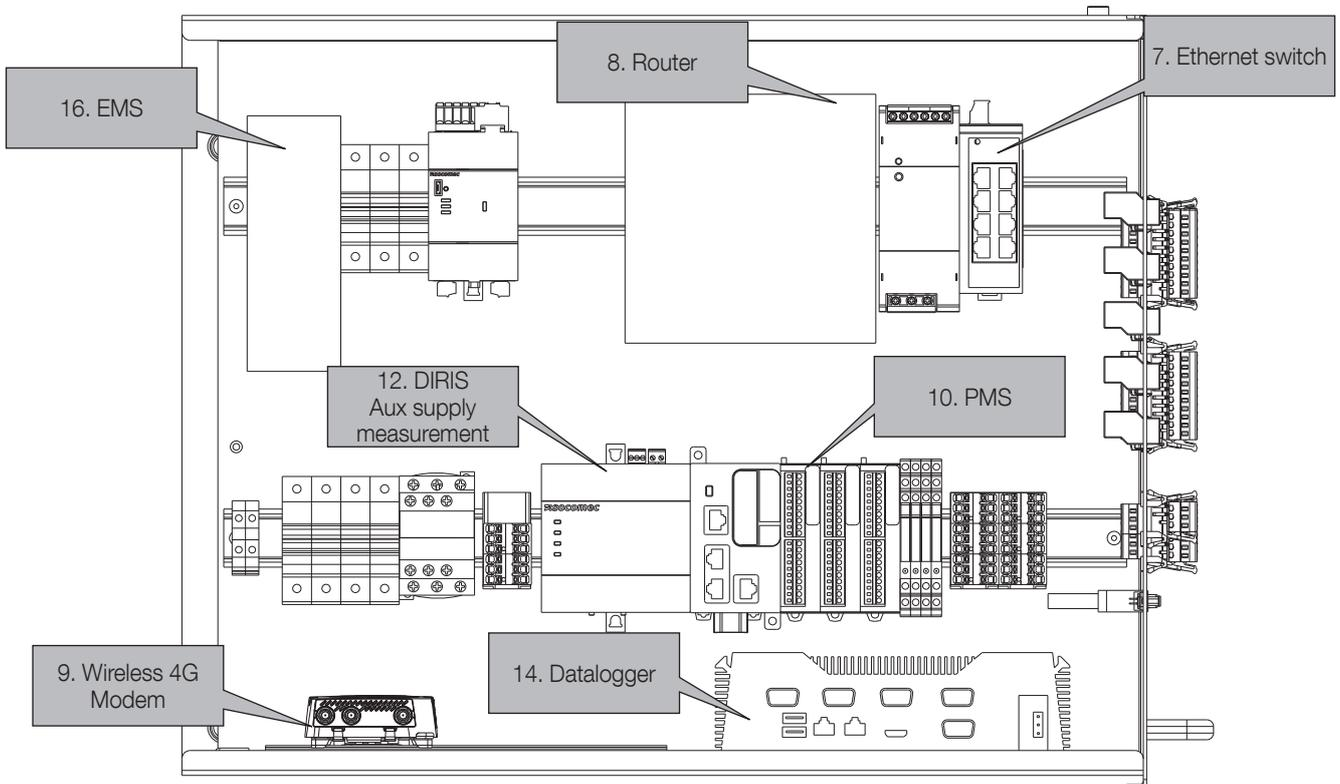
Figure 06. Detailed view of the Automation box
