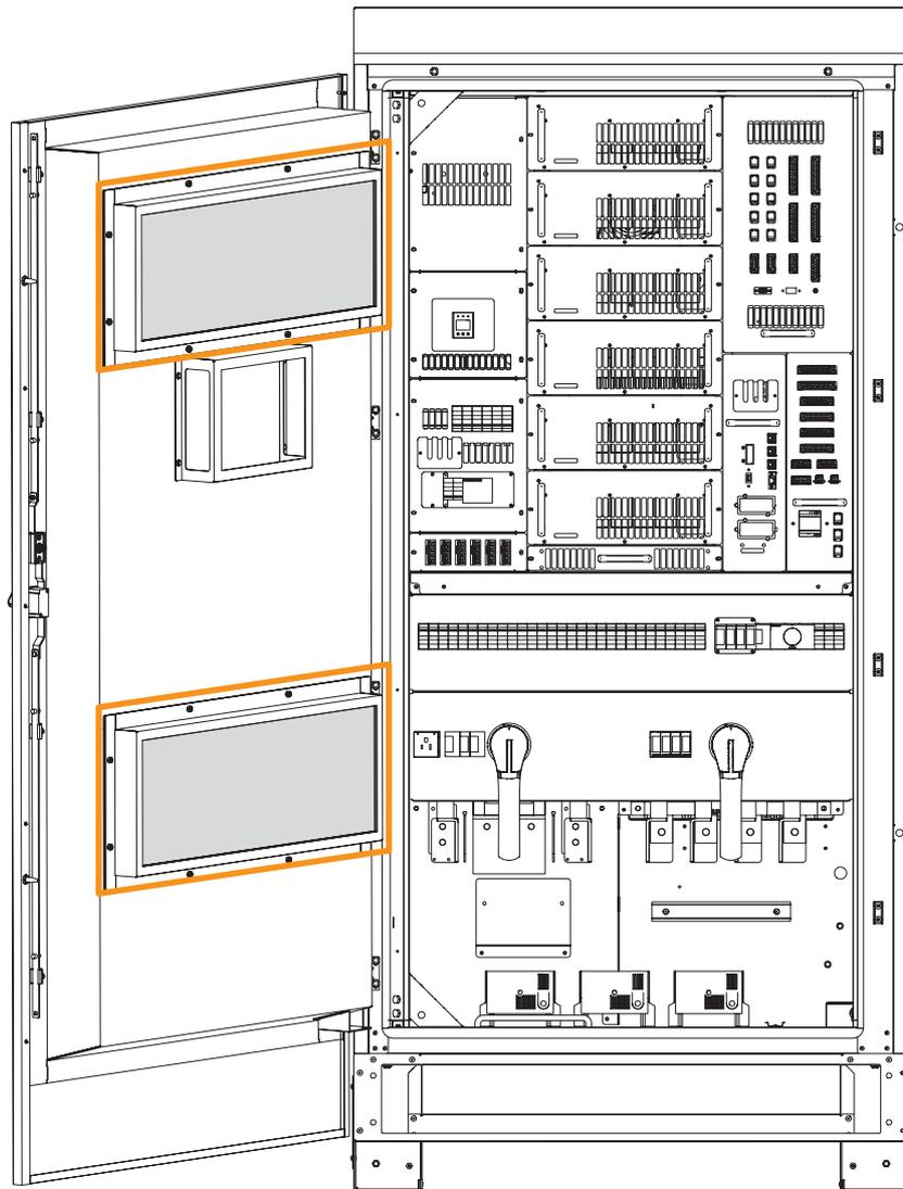
Figure 71. Location of the C-Cab air filters
