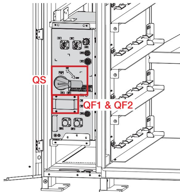
Figure 43. Location of isolation switch QS and breakers QF1 & QF2
