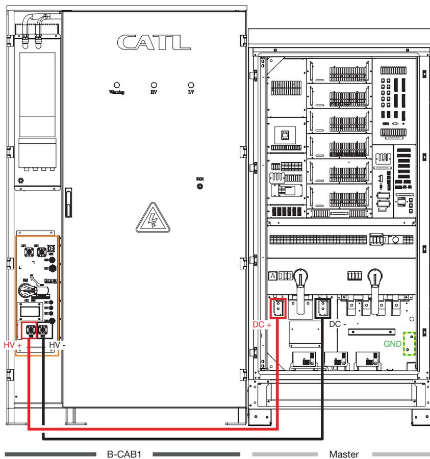
Figure 47. DC Power connections
