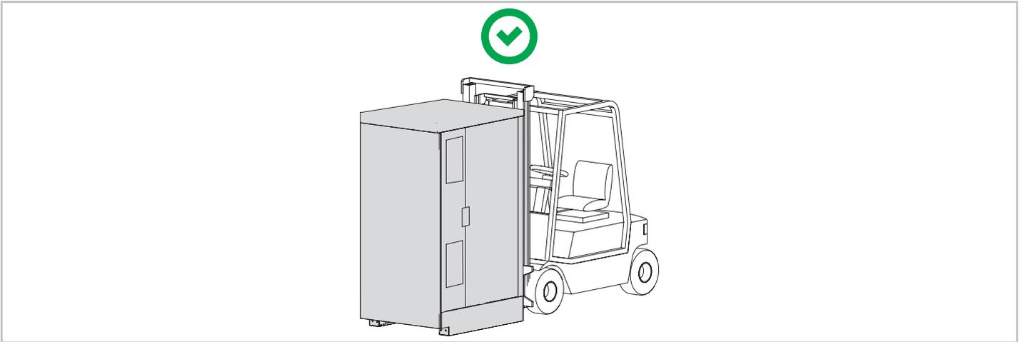
1. The forklift arm needs to be protected to avoid dirt pollution on the fork arm, or the forklift scrapes the bottom of the cabinet.
