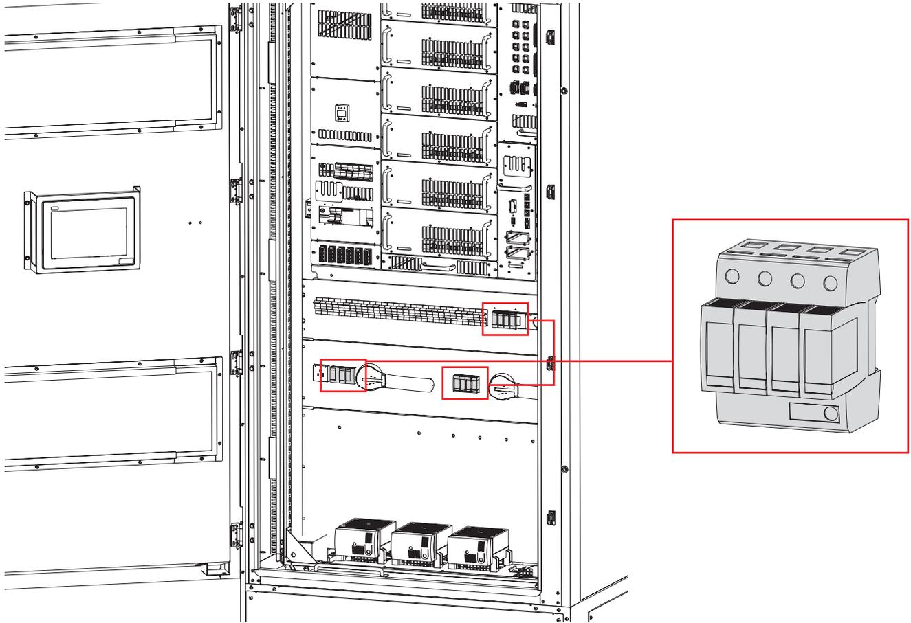
Figure 74. Location of the SPDs inside the C-Cab
