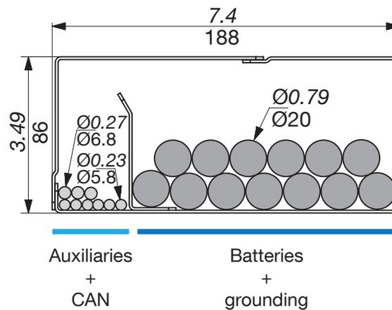
Figure 42. Cables organization inside the cable gutter
