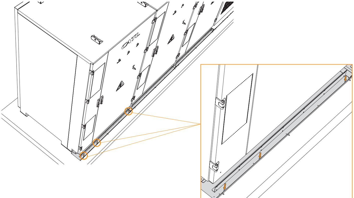
Figure 41. Cable connection kits locking
