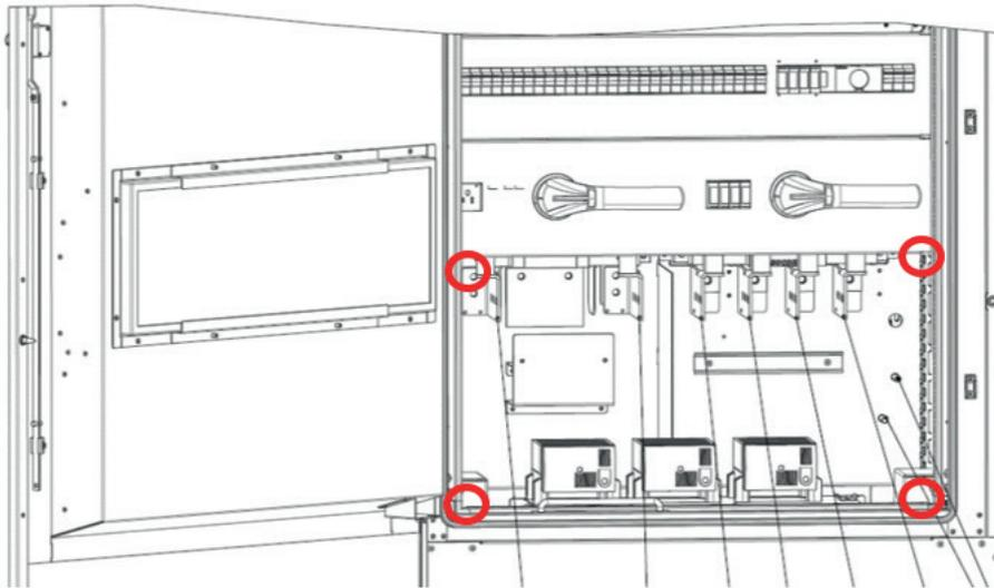
Figure 44. Screws of the plastic panel
