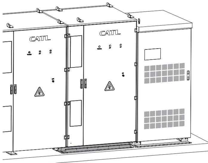
Figure 38. Installation of the B-Cab back part connection kit
