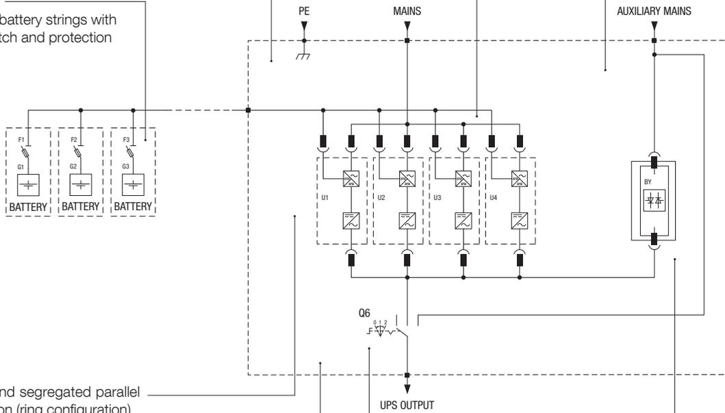
Redundant and segregated parallel bus connection (ring configuration)
