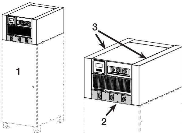
Installation on top of battery cabinets:
