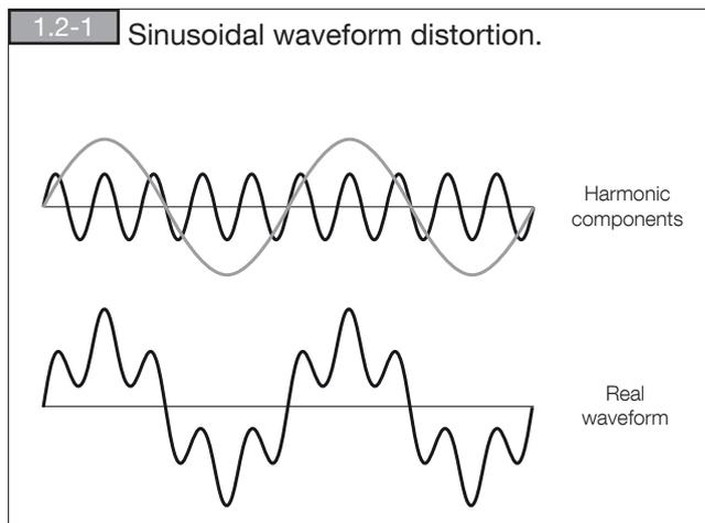
Harmonic currents circulating in the network cause voltage drops of the same order of magnitude and depending on the line impedance, with resulting voltage distortion.
