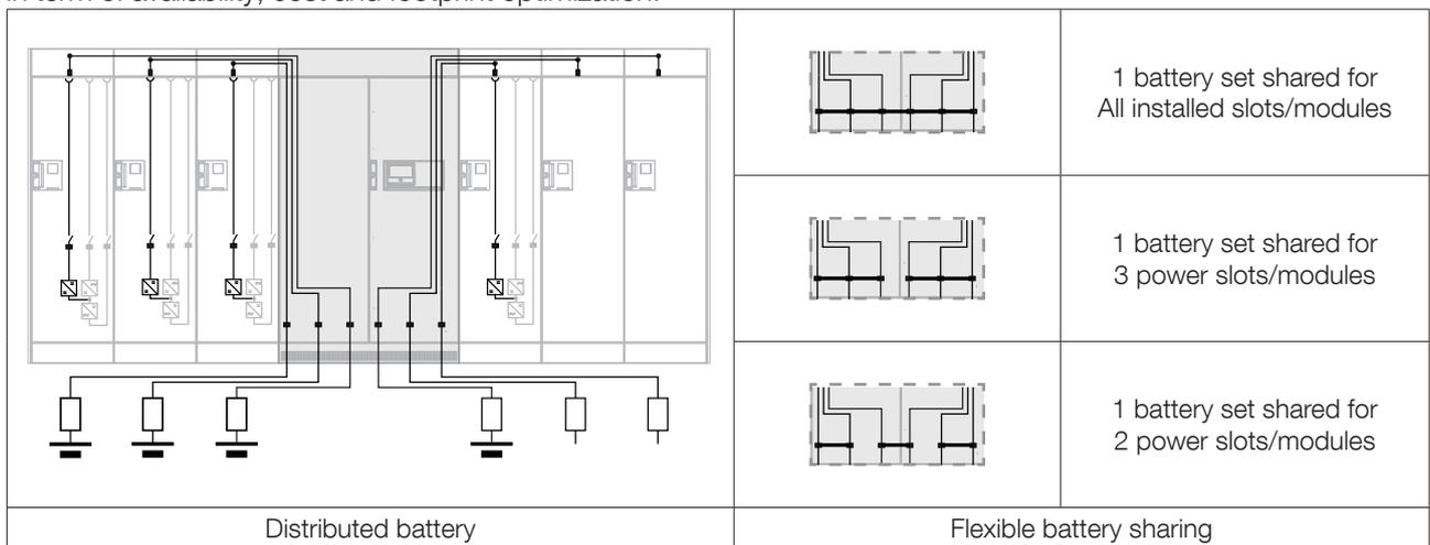
The battery switch in the module allows to connect / disconnect it from the battery bus without the need to remove the entire battery set (ie Shared battery).
