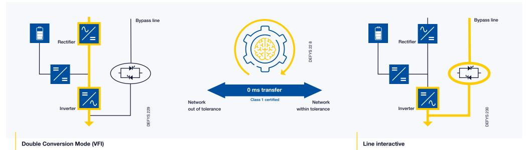
Inverters are always activated, taking the load instantaneously in double conversion in the event of grid disturbances.
