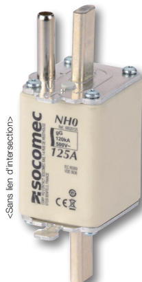
gG type fuse, NH0, with striker 16 to 200 A
