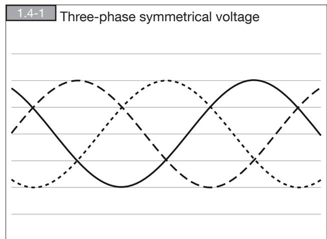
In general, even the nominal power of the transformers and the cable ratings are reduced in the case of significant asymmetry. In fact, the operating limit of these components is determined by the effective value of the total current which, in the case of imbalance, also consists of non-direct sequence currents. This fact must also be taken into account when adjusting the trip thresholds of protection devices which are sensitive to the total current.
