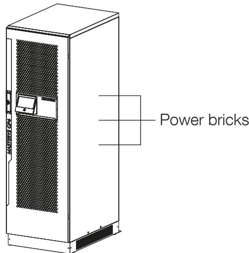
Any potential fault should be isolated inside the affected sub-assemblies, keeping the critical load protected in double conversion mode thanks to the remaining power converters to maximize the Mean Time Between Critical Failure.
