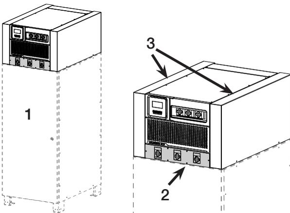
Installation on top of battery cabinets:
